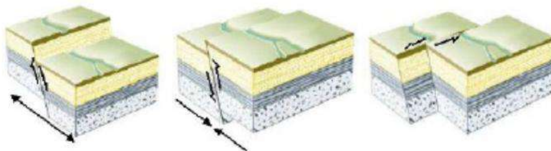
Figure 6-78: Normal Dip-Slip (left), Reverse Dip-Slip (middle) and Strike-Slip (right). Source: Hasan, Rahman, and Mahamud (2015)
