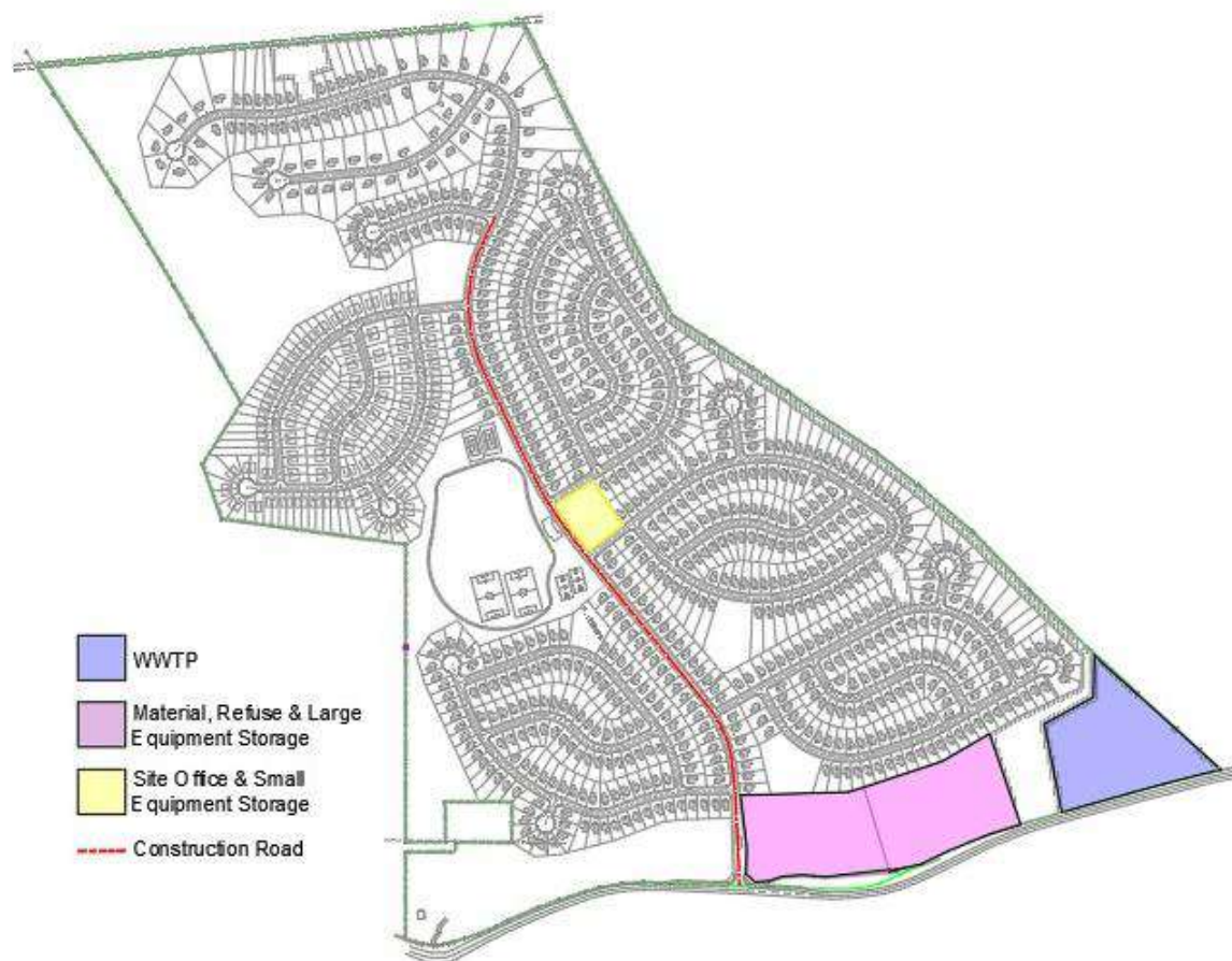
Figure 4-12: Diagram showing the location of the access road, site office and 'works yard' where aggregate material and equipment will be temporarily stored.
