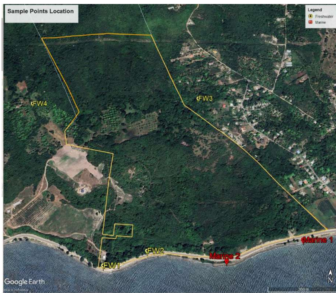
Figure 6-21: The location of the discharge and sample points (freshwater and marine) over the site and adjacent marine environment. It should be noted that the SCHIP road improvement project resulted in construction of drains that take runoff from the roadway into the sample environment, however, these were the only points accessible from land.
