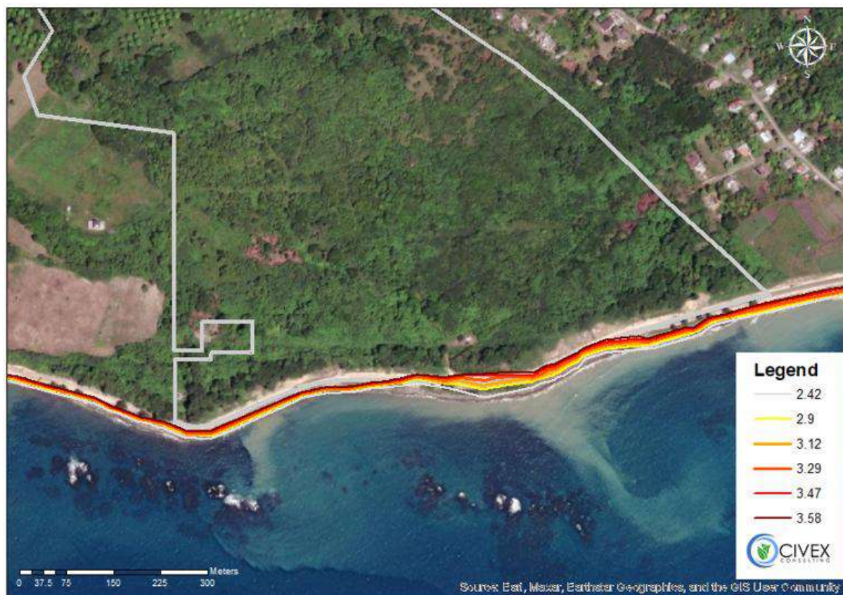
Figure 6-19: Approximate locations for each return period storm surge water surface elevation contour
