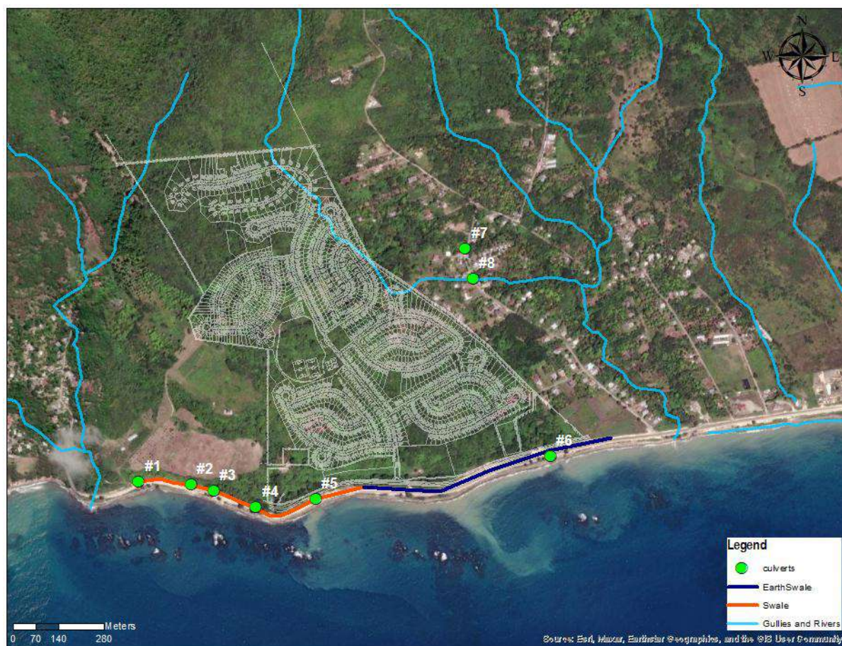
Figure 6-14: A map of the location of the existing drainage features within proximity of the proposed development
