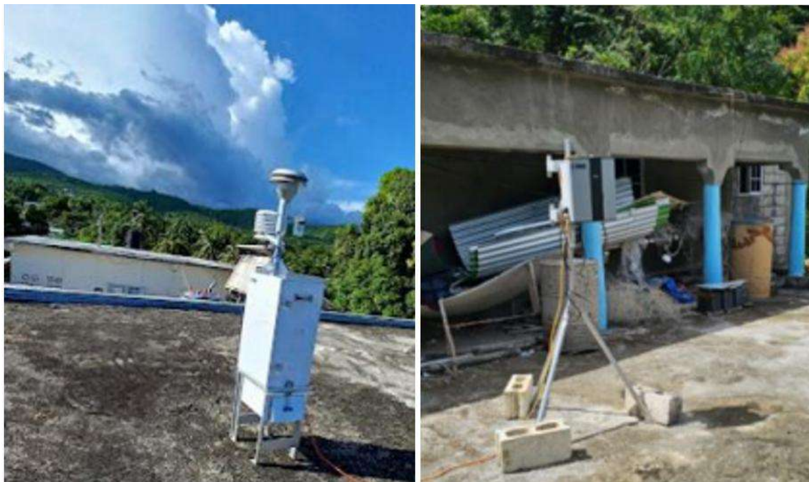
Figure 6-24: BAN-1022 on roof (upwind) while image on the left shows Polludrone on roof (downwind).
