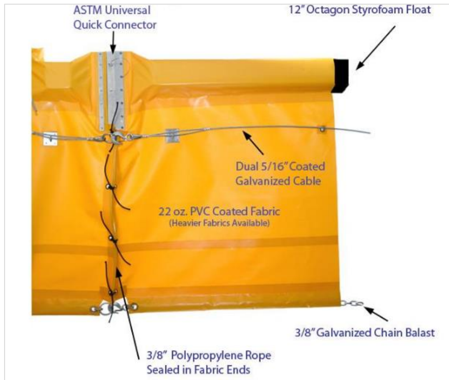
Figure 3-47 Specifications of a Mark III turbidity barrier
