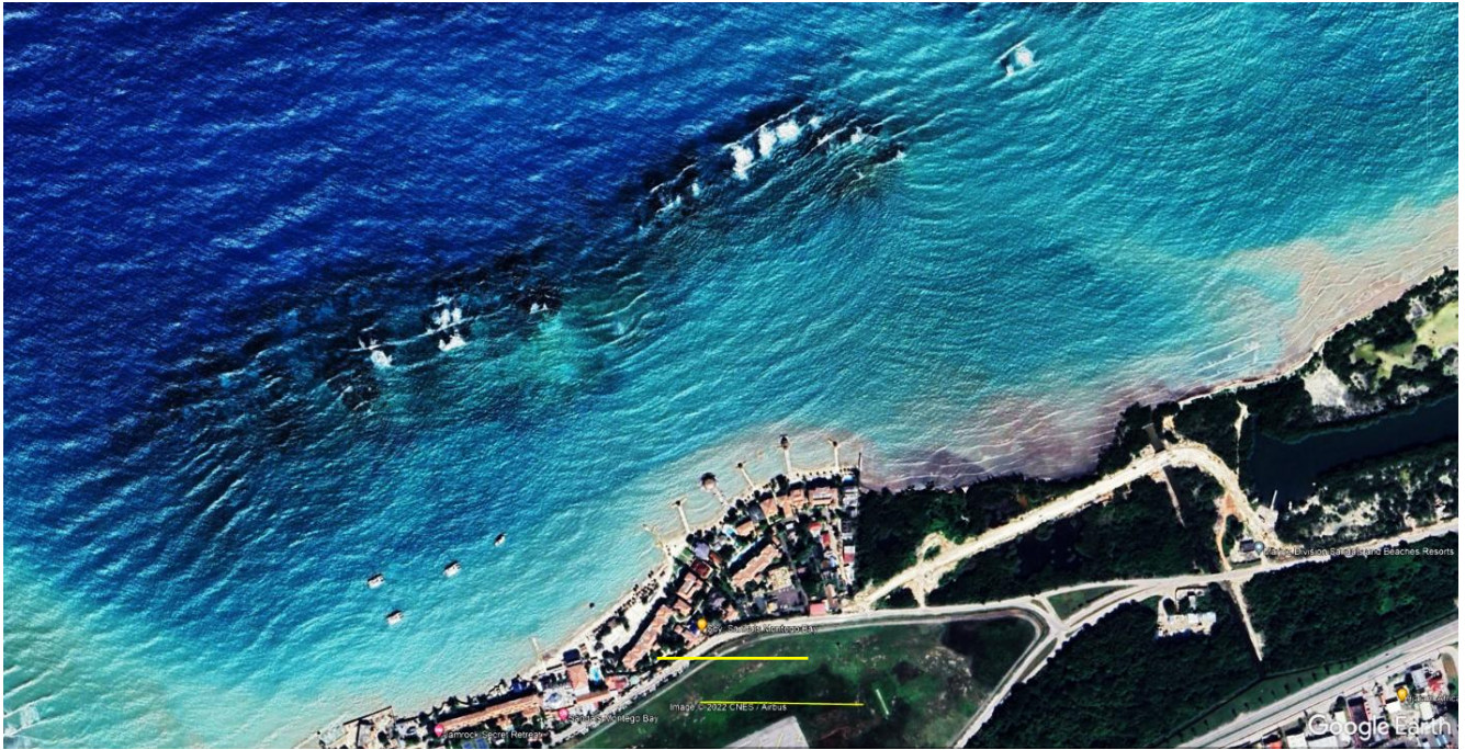
FIGURE 5-11: WAVE BREAKING OVER THE SHALLOW BARRIER REEF AND WAVE PROPAGATION THROUGH THE GAPS . YELLOW LINE = 200 M.
