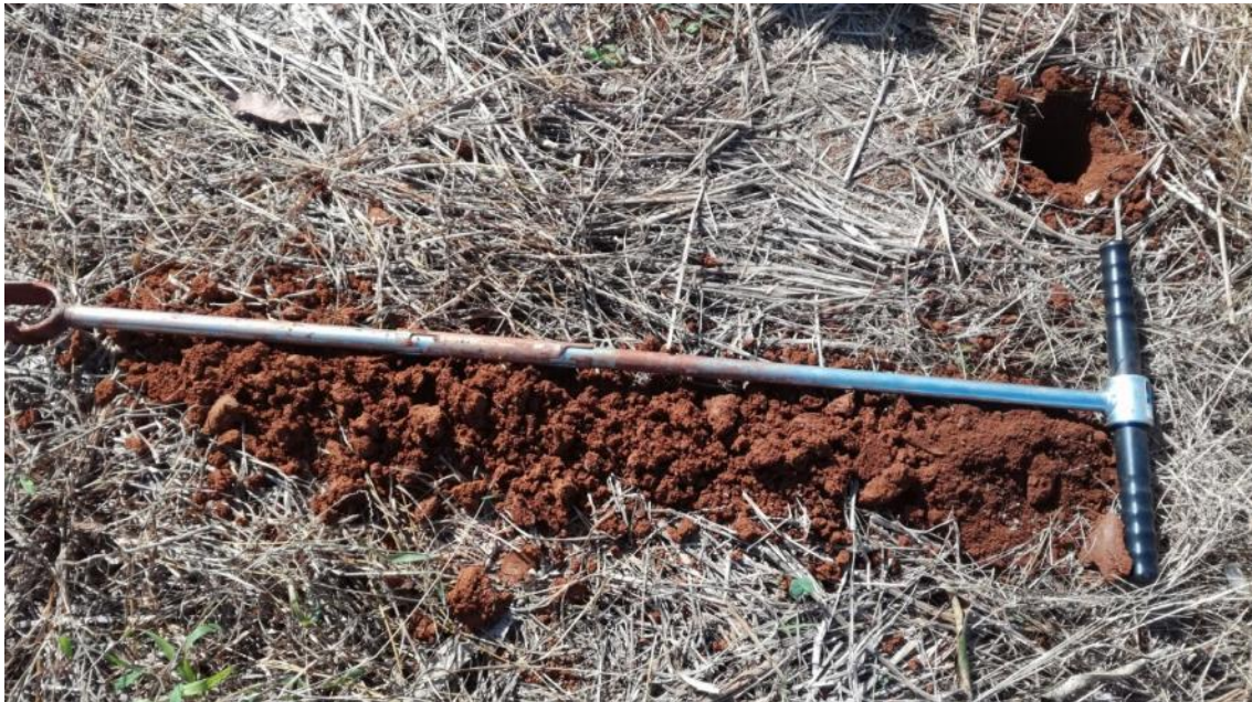
Picture 20 - Survey J1 red soil, slightly acidic pH, thick soil without pebbles under mulch and cultivation of beetroot
