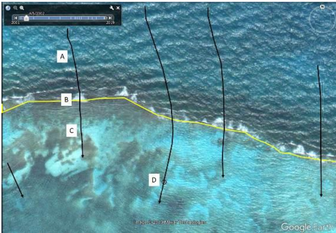
Figure 6J-1: Google Earth Image Dated April 5, 2002 Depicting Wave Movements Apparently Driven By Winds Blowing Out Of The North Northwest (A-areas between 1-9m depth, B-reef area between 0.3m-1m, C-areas between 0.3m-1.8m, D-project location).
