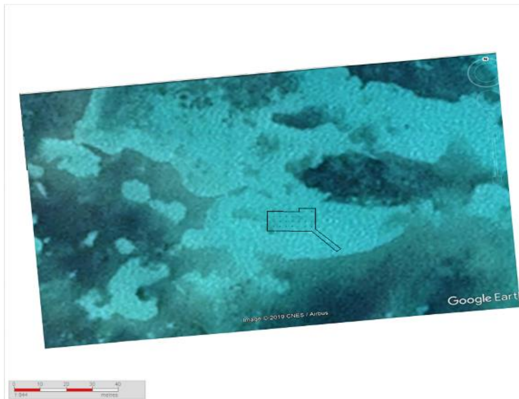
Figure 5B: Pile Layout Superimposed onto Google Earth Image of Proposed Site At Lilliput (relate to Figure 1B)
