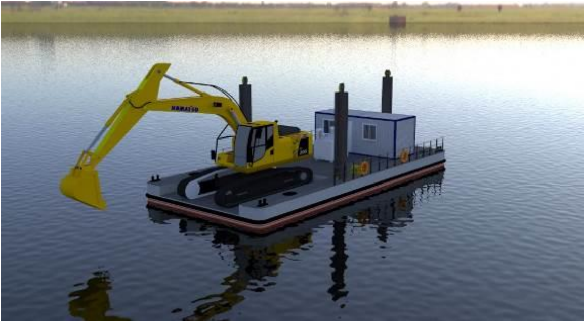
Plate 8A: 32 Illustration of a 3-Spud Work Barge (the barge depicted shows an excavator, however, for this project, a pile driver will be the supported equipment).
