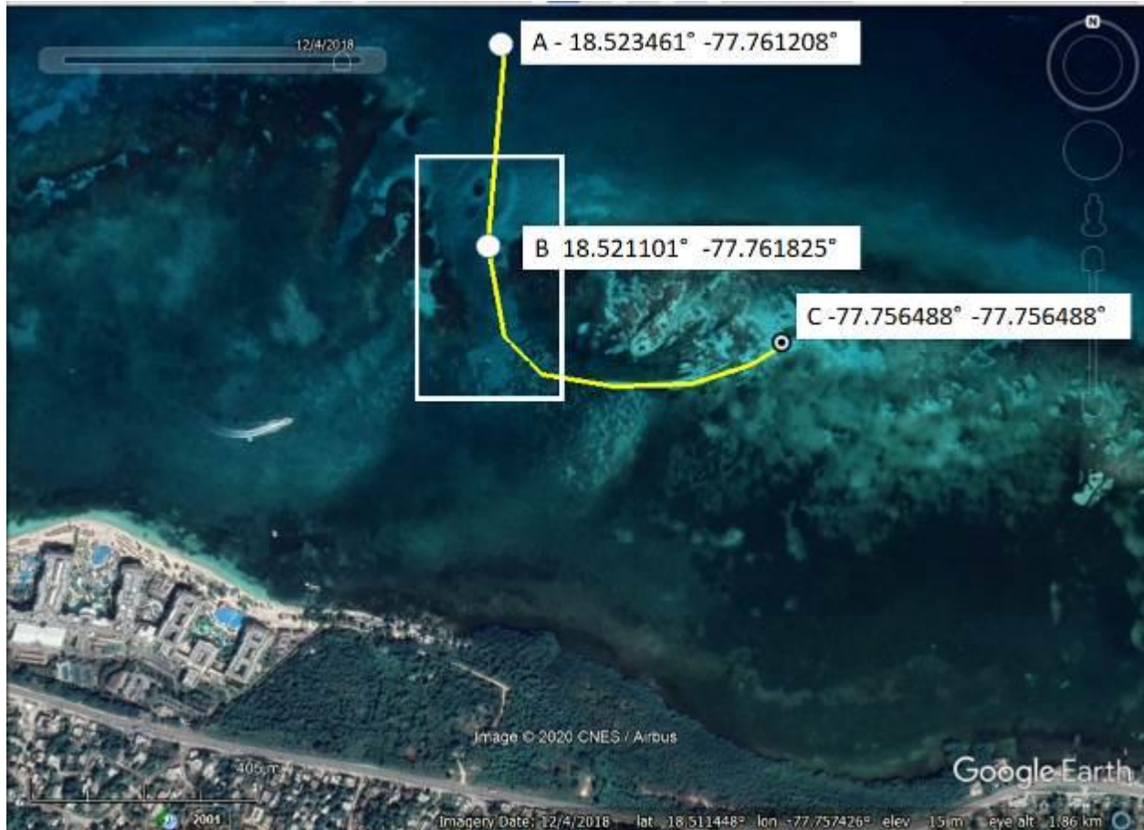
Figure 6Q: Proposed Access Path for A Work Barge Being Towed To The Work Site (A: approach pathway, B: access through reef, C: worksite location).
