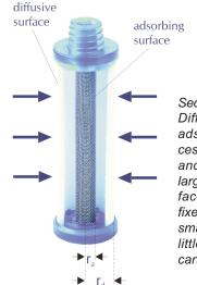
Section of radiello. Diffusive and adsorbing surfaces are cylindrical and coaxial: а large diffusive surface faces, at a fixed distance, the small surface of a little concentric cartridge.
