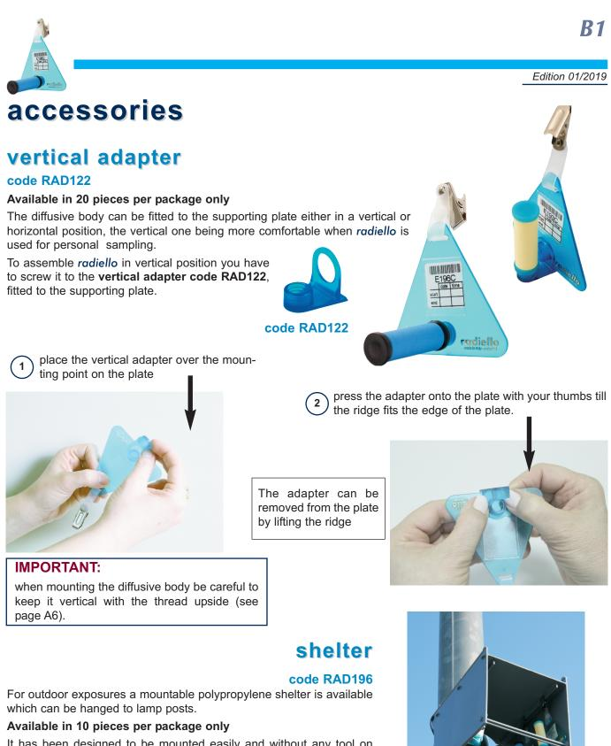
It has been designed to be mounted easily and without any tool on field, so that it is not cumbersome when you transport it from your laboratory. Once assembled, it ensures the best compromise between protection against bad weather and ventilation.
