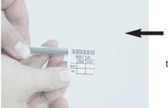
Keep note of the date and time of the end of exposure. Place the cartridge into the tube, peel off the label and stick it onto the tube <u>such that the barcode is parallel to the axis of the tube</u>.
