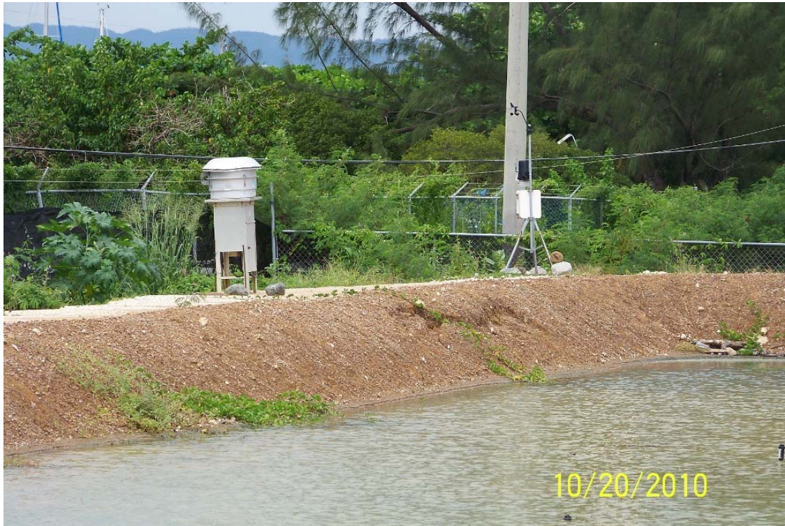
Plate 11 Photo showing ambient air sampler and weather station
