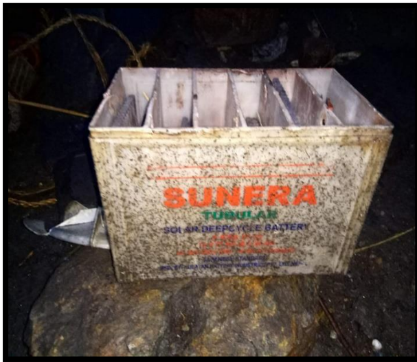
Figure 5: Plastic housing for a used lead acid battery that would have been contaminated by the lead and acid content of the battery is presumed to be hazardous. Lead is a constituent of Annex I that results in toxicity, and the acid in the battery is corrosive. Both are characteristics of Annex III.
