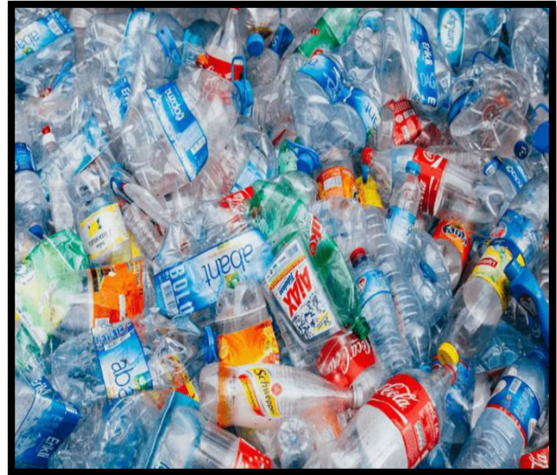
Figure 9: Polyethylene Terephthalate (PET) plastic beverage bottles that are almost free from contamination and other types of
