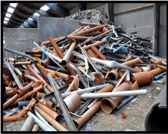
Figure 1: Polyvinyl Chloride (PVC) pipes, gutters and cable trays some of the plastics covered under the Y48 entry.
