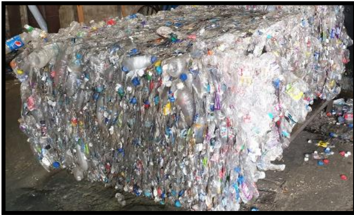
Figure 12: Baled Polyethylene Terephthalate (PET) clear plastic beverage bottles with polypropylene caps. The bale had signs of contamination.
