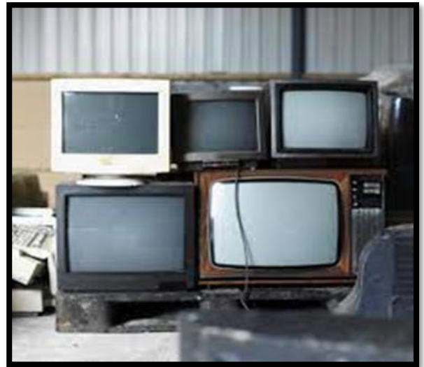
Figure 6: Television and computer monitors are made of plastics that contain flame retardants, made of brominated compounds. Bromine is a constituent of Annex I with Annex III characteristics. The plastic housings are hazardous plastic waste classified as entry A3210 of Annex VIII.
