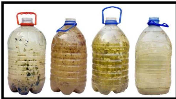
Figure 3: Polyethylene terephthalate (PET) bottles that are not free of contamination and are significantly dirty. Similar to the state of plastic waste removed from the disposal site or a blocked gully.
