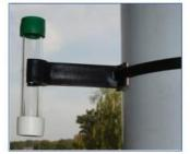
**Description:** Acrylic tube fitted with a green and white thermoplastic rubber caps. The green cap contains the absorbent and the white cap is fitted with a filter to prevent the ingress of particulates. This tube is designed to simultaneously passively monitor gaseous NO<sub>2</sub> and SO<sub>2</sub>. Analysis of exposed tubes is carried out by Ion Chromatography (UKAS Accredited Methods).
