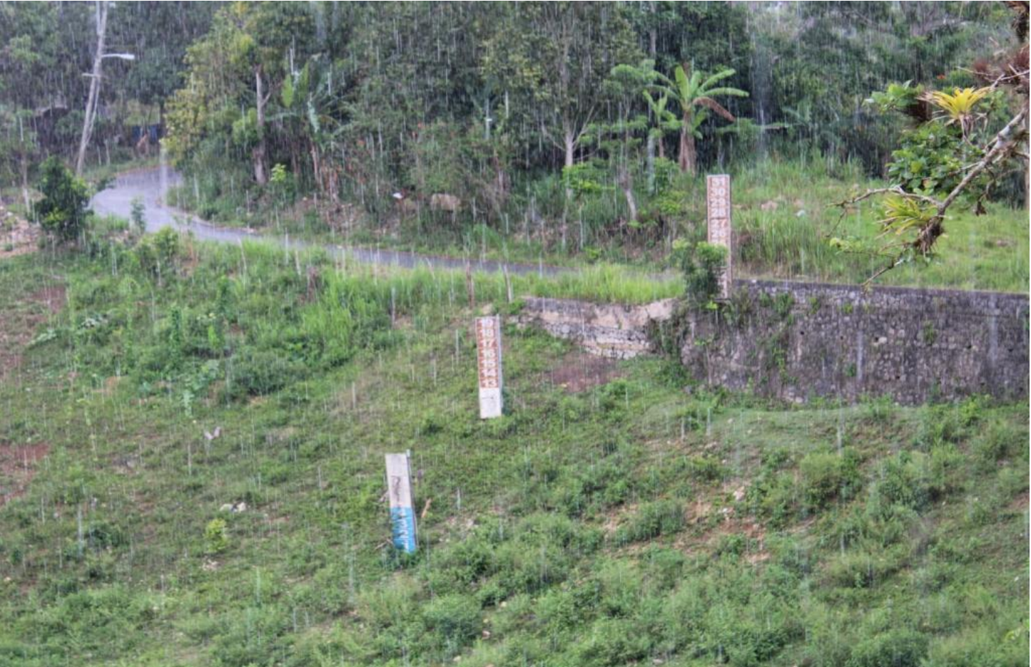
Plate 145: A basin which is equipped with rain gauges for measuring the rainfall when flooding occurs
