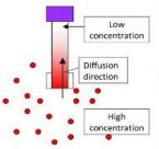
Diffusion tubes work by a process called molecular diffusion. During molecular diffusion, compounds will move from an area of high concentration to an area of low concentration.
