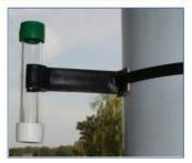
**Description:** Acrylic tube fitted with a green and white thermoplastic rubber caps. The green cap contains the absorbent and the white cap is fitted with a filter to prevent the ingress of particulates. This tube is designed to simultaneously passively monitor gaseous  $NO_2$  and  $SO_2$ . Analysis of exposed tubes is carried out by Ion Chromatography (UKAS Accredited Methods).
