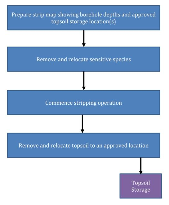
Figure 4-3: Process flowchart for Site Clearance for each orebody
