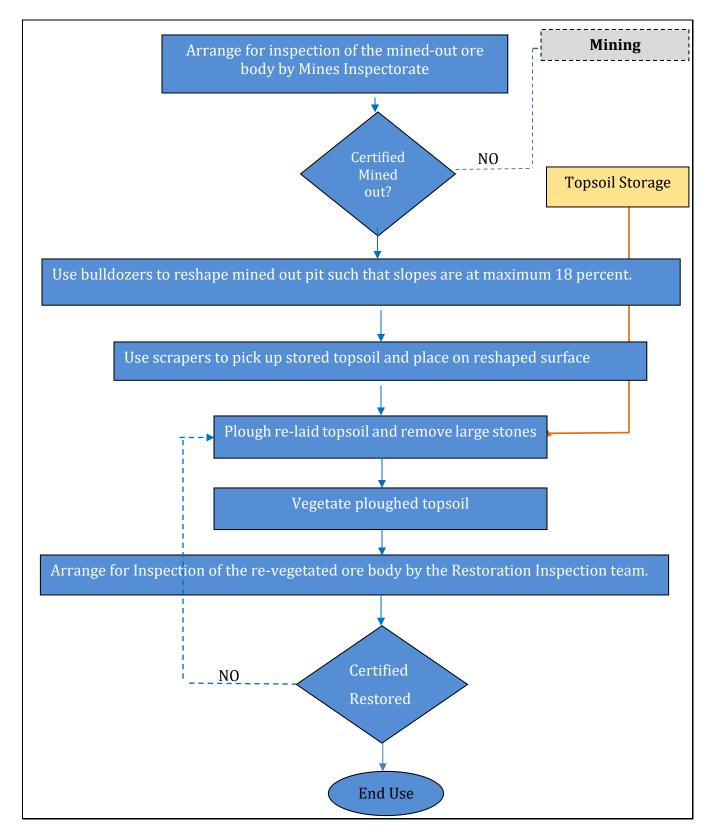
Figure 4-6: Process Flow for Rehabilitation of mined out areas
