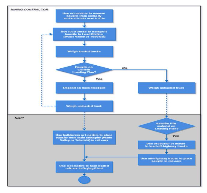
Figure 4-5: Flowchart of mining process
