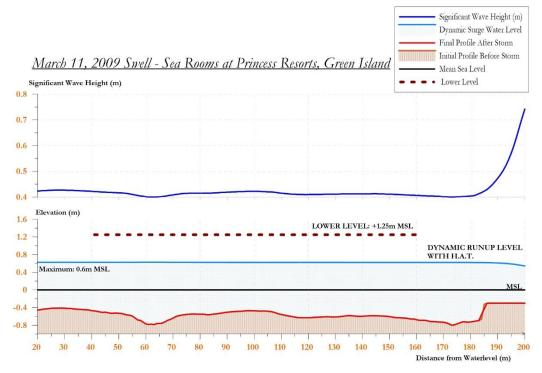
Figure 8.6 Water elevation along the footprint of the Sea Rooms under swell conditions
