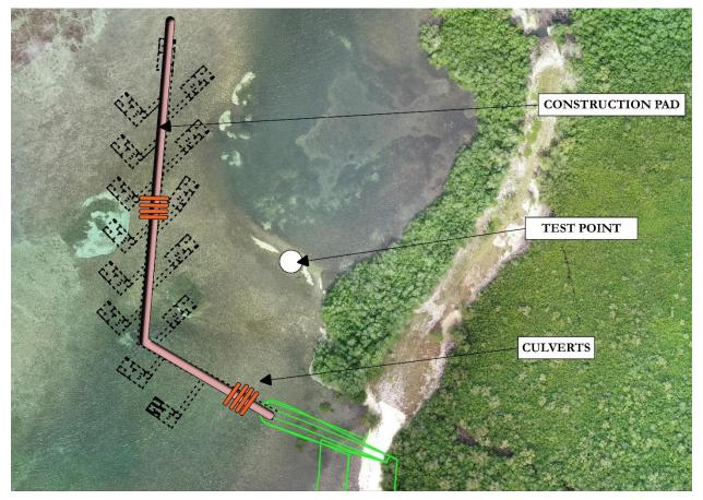
Figure 9.1 Schematic showing the layout of construction pad and culvert
