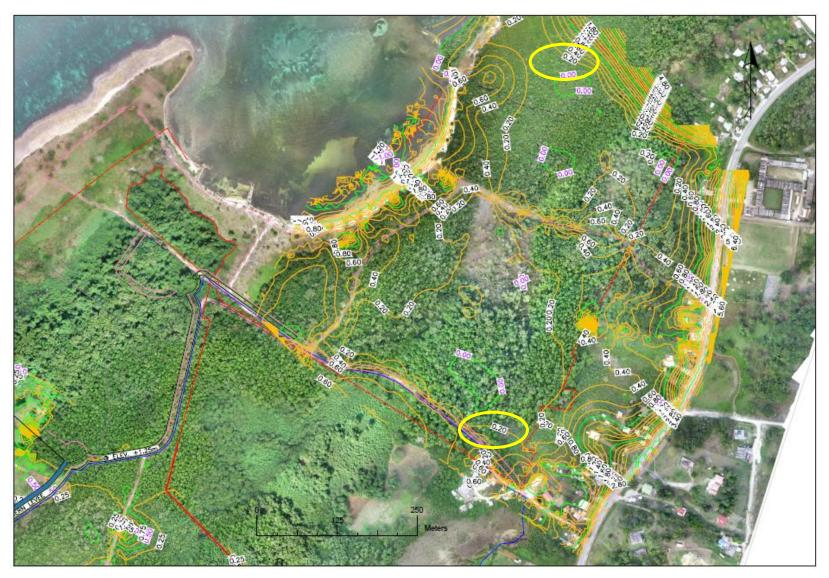
Figure 1.7: Topographic results for eastern end of property, highlighting identical elevations in forest (yellow circles) and degraded mangrove area (Rehab#1)
