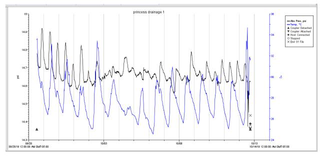
Figure 1.9: Water level logger results for western drainage pond area periphery
