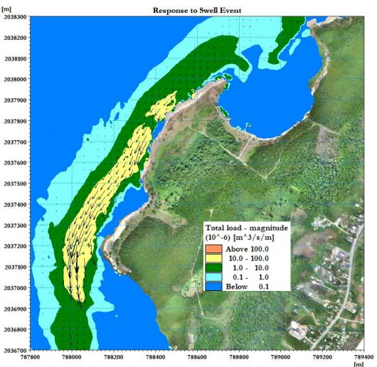
Figure 5.21 Total amount of suspended sediments and the direction of flow at the peak of the swell event
