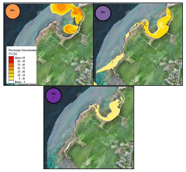
Figure 9.3 Flushing provided by two 15m wide culverts
