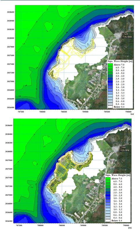
Figure 7.9 Significant wave heights under the 1 in 50-year event with no structures in place (top) and with structures in place (bottom)
