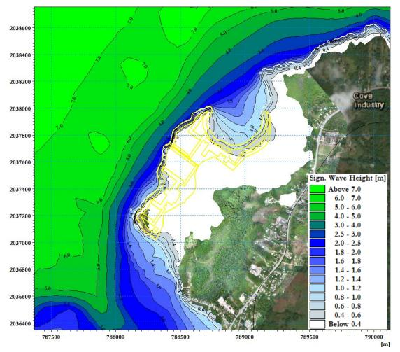
Figure 5.12 Significant wave heights under the 1 in 50yr hurricane condition
