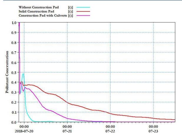
Figure 9.2 Flushing potential with and without the construction pad at the test point shown above
