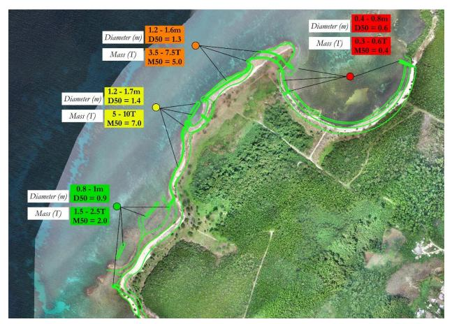
Figure 8.4 Stone sizes at the sections of the site
