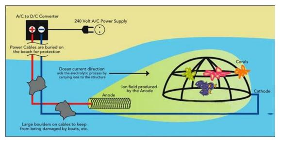
Figure 9.8 Schematic of coral reef electrification process
