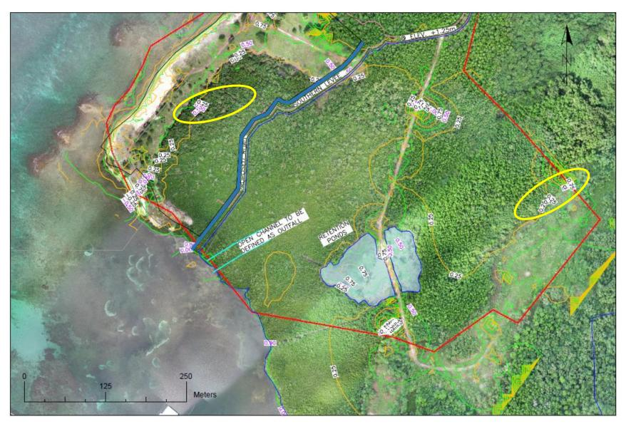
Figure 1.6: Western mangrove topography with proposed drainage ponds
