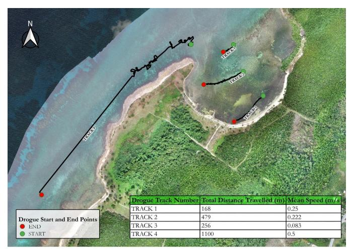
Figure 2.12 Current measurement with the drogue
