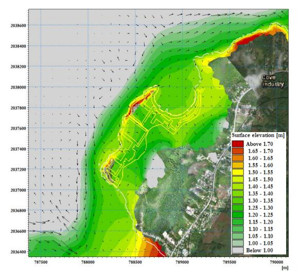
Figure 5.11 Static water level above MSL under the 1 in 50yr hurricane condition
