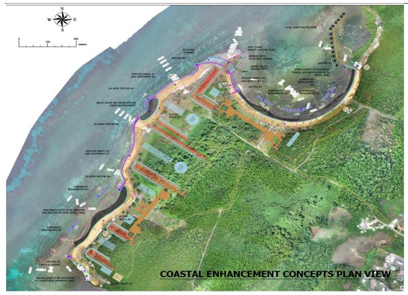
Figure 1.1 Site plan of proposed coastal enhancement works at Princess Resort, Hanover
