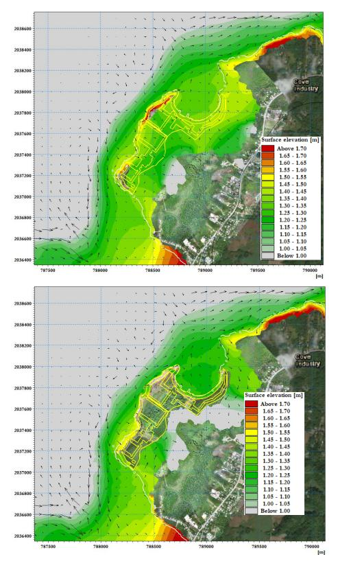
Figure 7.8 Static storm surge levels (50-year event) with no structures in place (top) and with structures in place (bottom)
