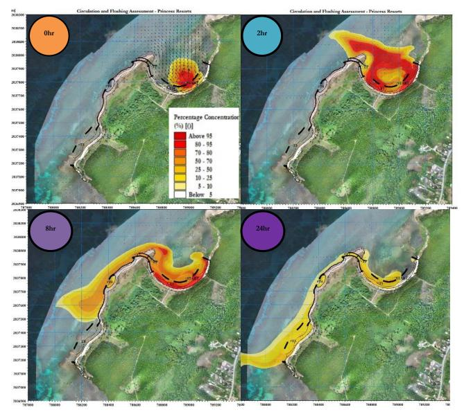
Figure 7.2 Flushing conditions after 24 hours with the introduction of a pollutant in Proposed Conditions
