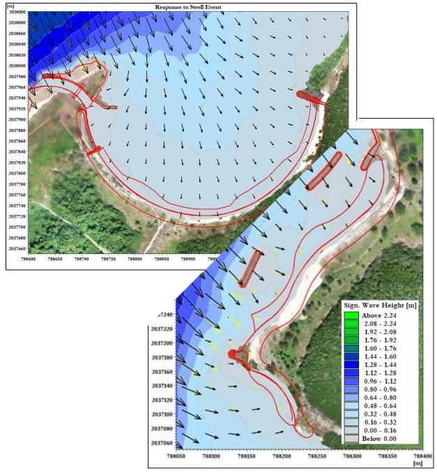
Figure 7.4 Swell wave response at the Hotel 1 and 4 (Yellow Arrows Proposed Conditions – Black Arrows Existing Conditions)
