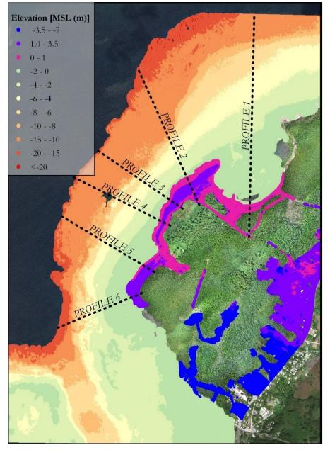
Figure 2.8 Collation of nearshore and terrestrial elevation points referenced to mean sea level (MSL)
