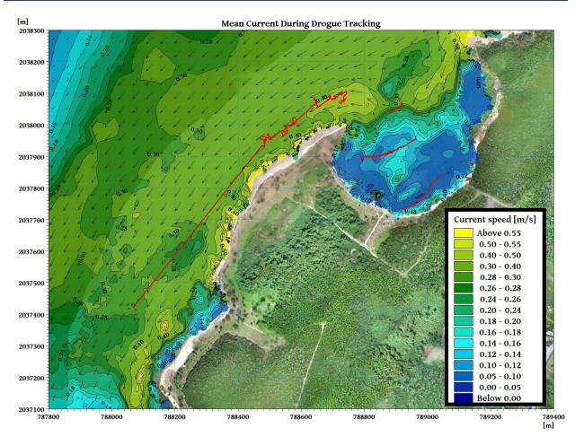
Figure 5.3 Mean current speed during the drogue measurement period
