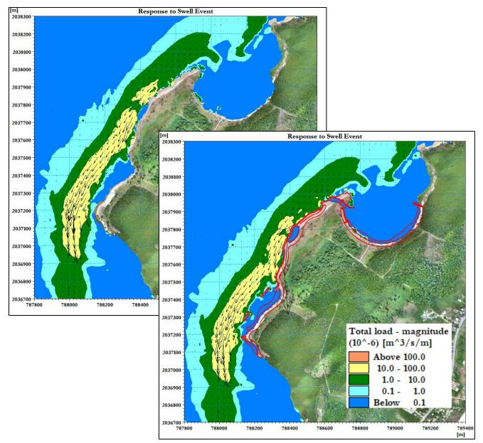
Figure 7.7 Potential total suspended sediment in existing and proposed conditions at the peak of swell
