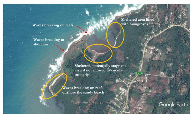
Figure 2.2 Aerial image of site showing waves breaking on reefs along the shoreline
