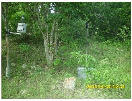
Plate 4-4 Noise (right) and particulate (left) meter
