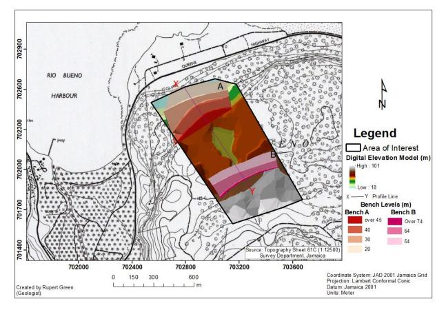
Figure 3-17 Digital Elevation Model (DEM) overlain on topographic map for the area of interest showing terracing configuration after preliminary operations
