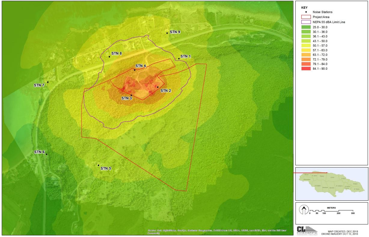
Predicted noise emissions from the quarry operations using ISO 9613-2: 1996 Prediction Method Figure 6-9
