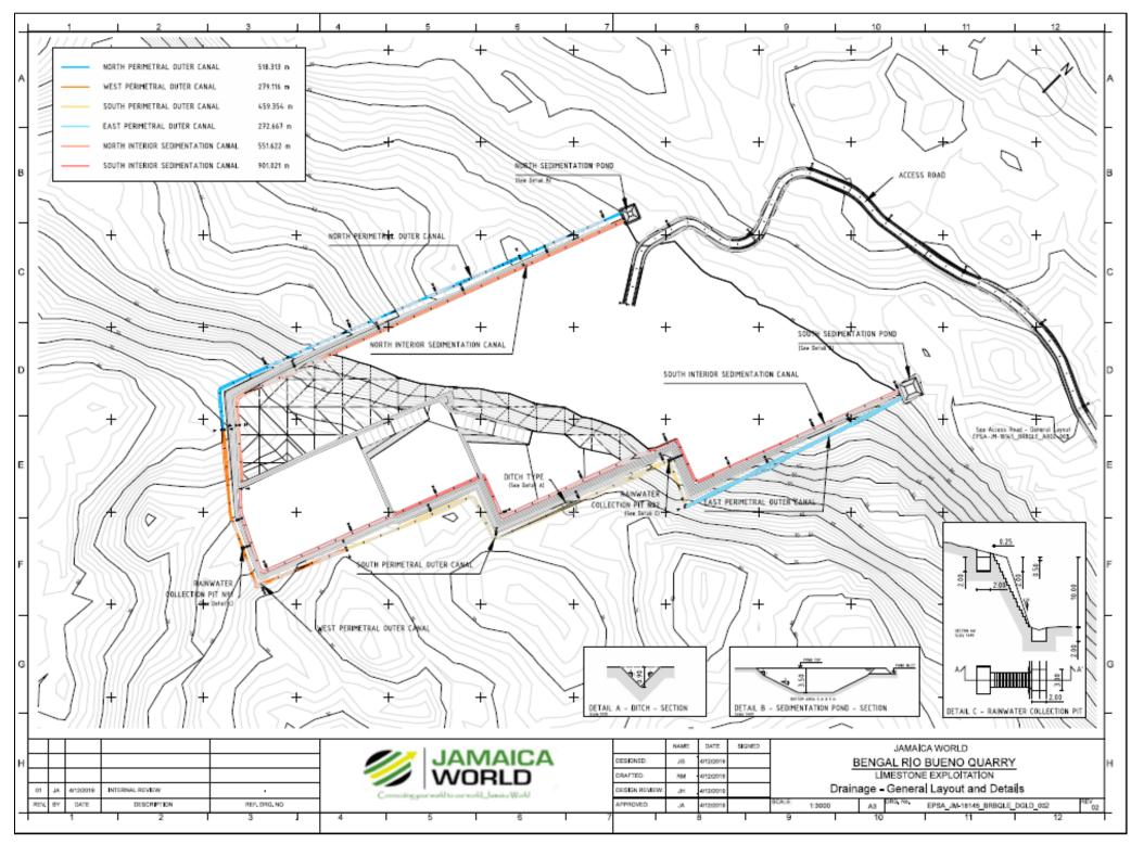
Figure 3-4 Drainage Layout for quarrying facility
