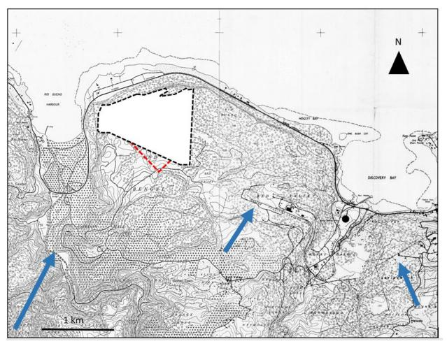
Figure 4-8 Topographic map showing regional groundwater flow directions for the area (blue arrows). White area outlines the proposed quarry site (Source: JAD 1:12,500, WRA)
