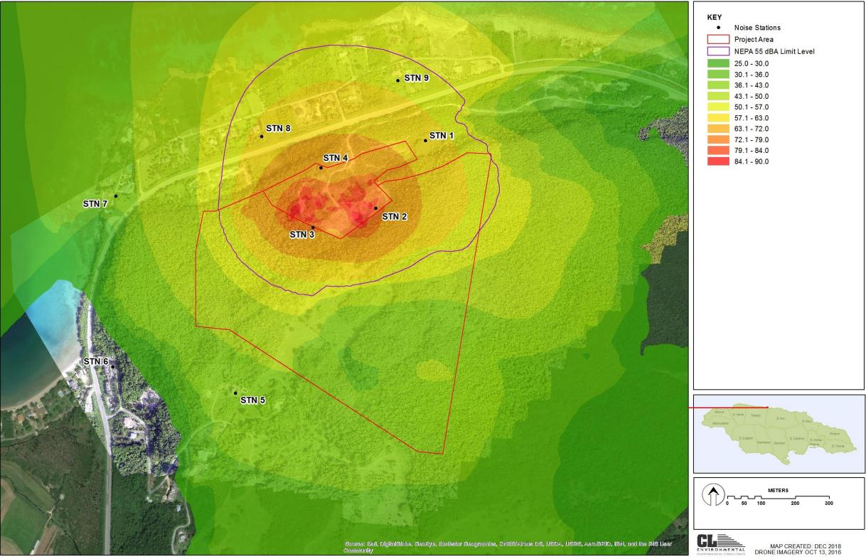
Figure 6-10 Predicted noise emissions from the quarry operations using Concawe Prediction Method (wind from the southwest)
