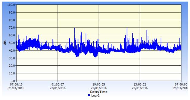
Figure 4-33 Noise fluctuation (Leq) over 72 hours at Station 4
