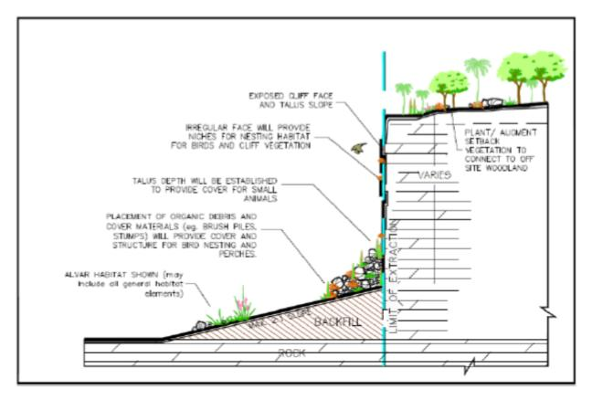
Figure 3-22 Sideslope Detail (talus slope and exposed cliff face)
