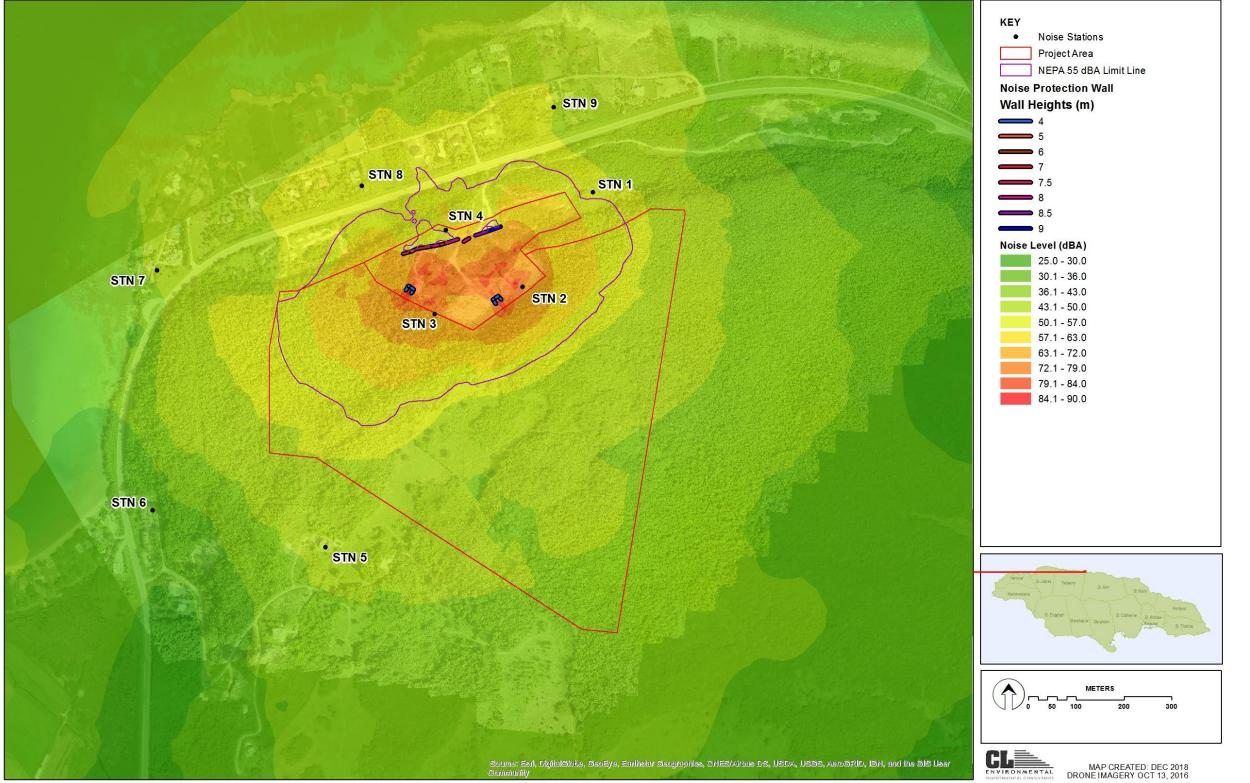
Predicted noise emissions from the quarry operations with mitigation using ISO 9613-2: 1996 Prediction Method Figure 6-11
