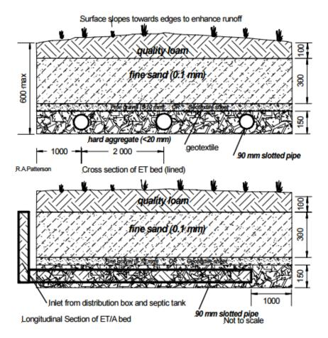
Figure 3-8 Cross and longitudinal section of evapotranspiration bed
