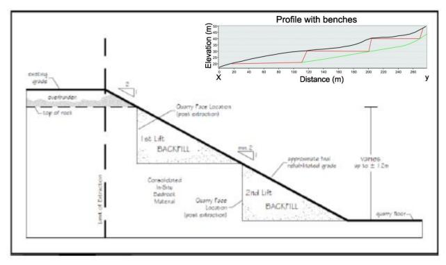
Figure 3-23 Quarry Profile vs Reclaim Slope with Backfill
