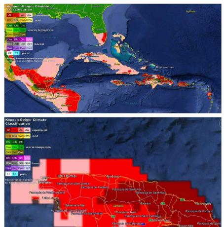
Because the quarry is located in a storm zone (Am – Tropical Monsoon), we are going to consider an extreme case in which all the precipitation of a month fell in the form of a storm in one hour. In this way we ensure that the drainage system is able to work correctly for any possible situation.
