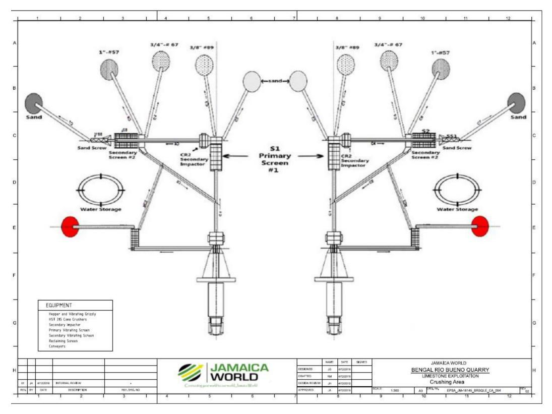
Figure 3-10 Crushing area equipment each with a water storage tank
