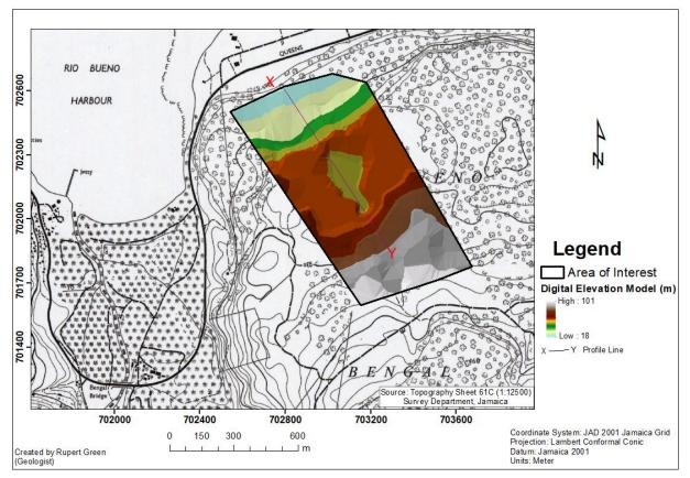
Figure 3-14 Digital Elevation Model showing cross section for bench design
