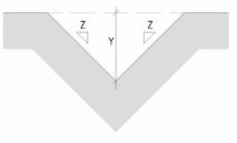
The drainage capacity of the ditch can be calculated using the following Manning's formula:
