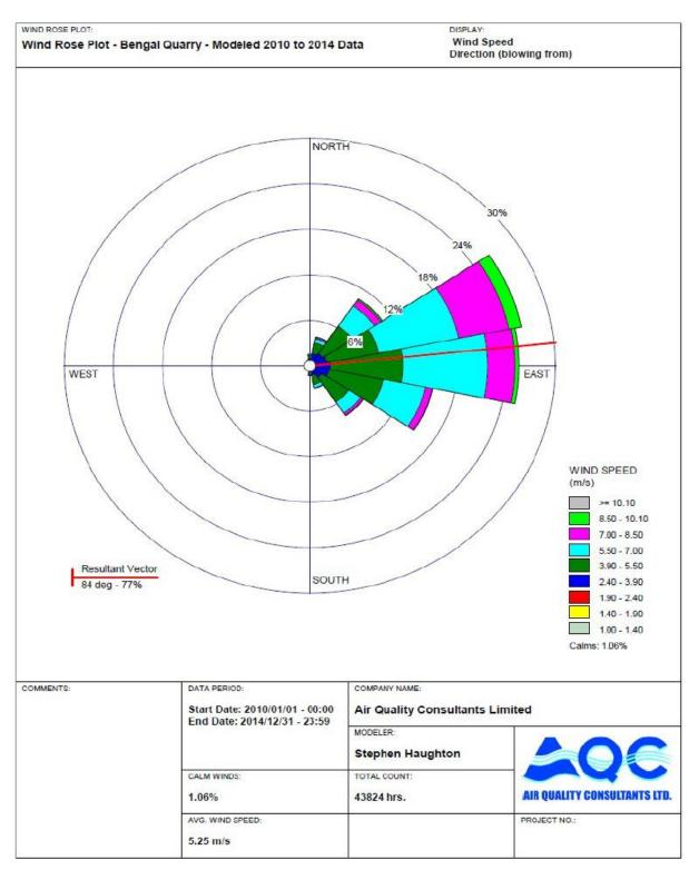
Figure 6-2 Wind Rose Plot – 2010-2014 Modeled Met Data for Proposed Quarry Site
