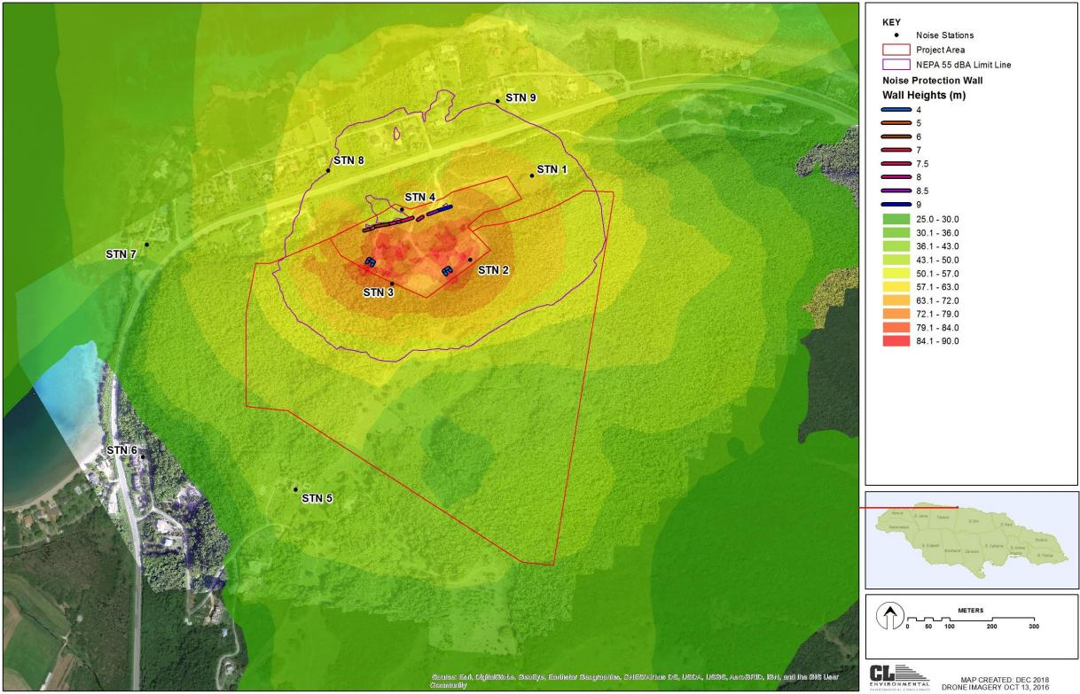
Predicted noise emissions from the quarry operations with mitigation using Concawe Prediction Method (wind from the southwest) Figure 6-12
