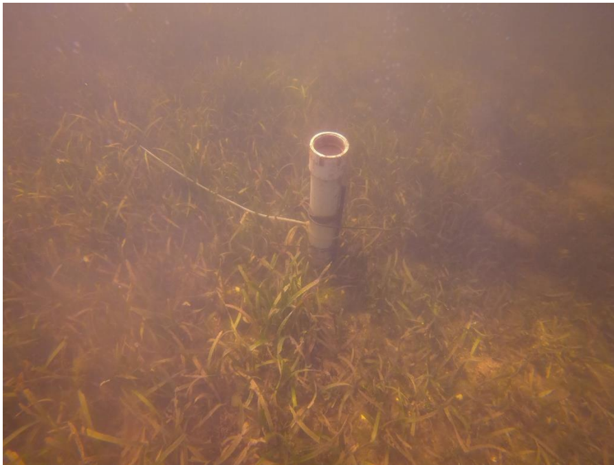
Plate 6-4 Sediment Trap deployed nearshore at Station S5
