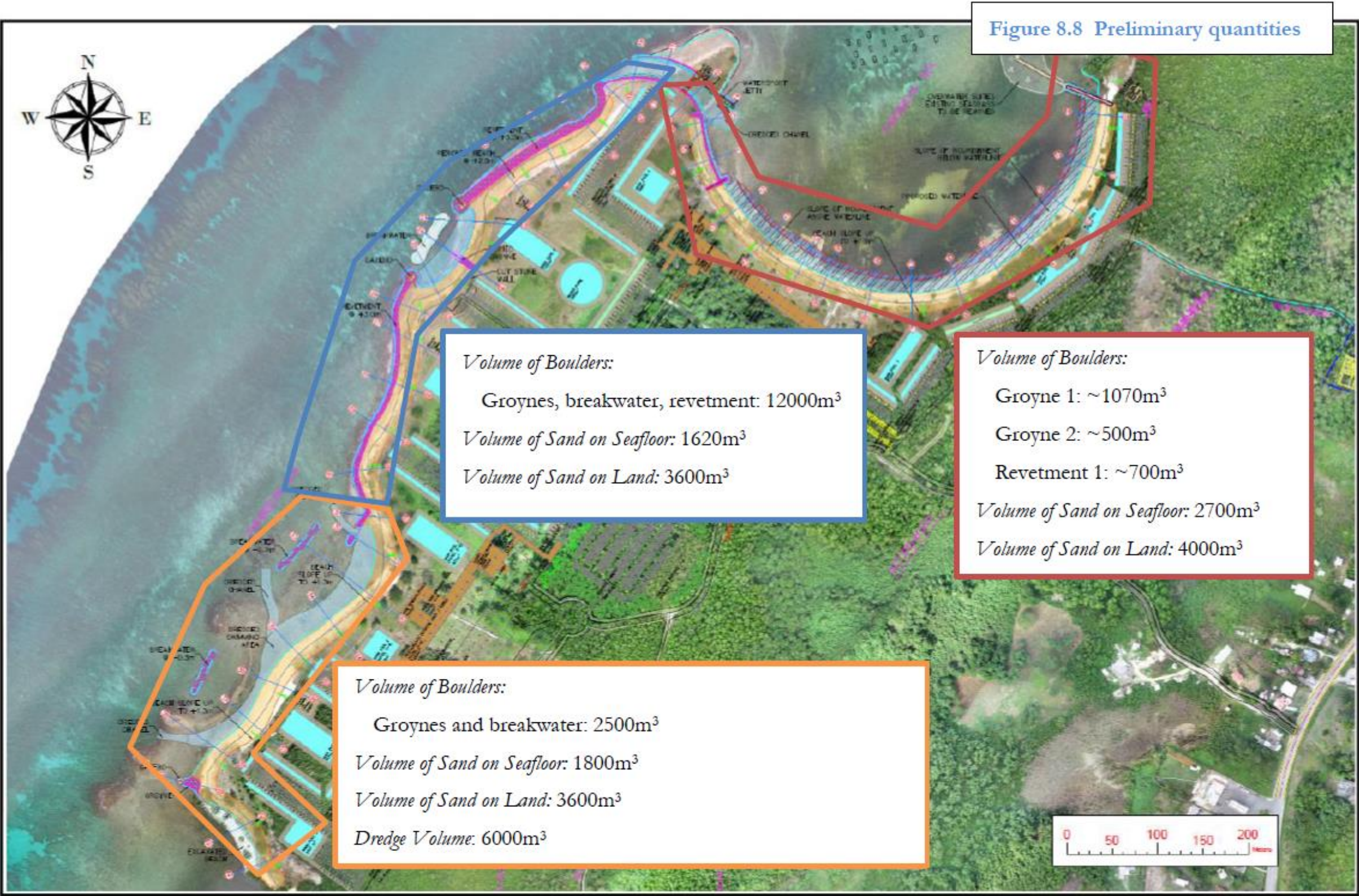
Figure 5-28 Preliminary quantities of boulders and sand for beach works
