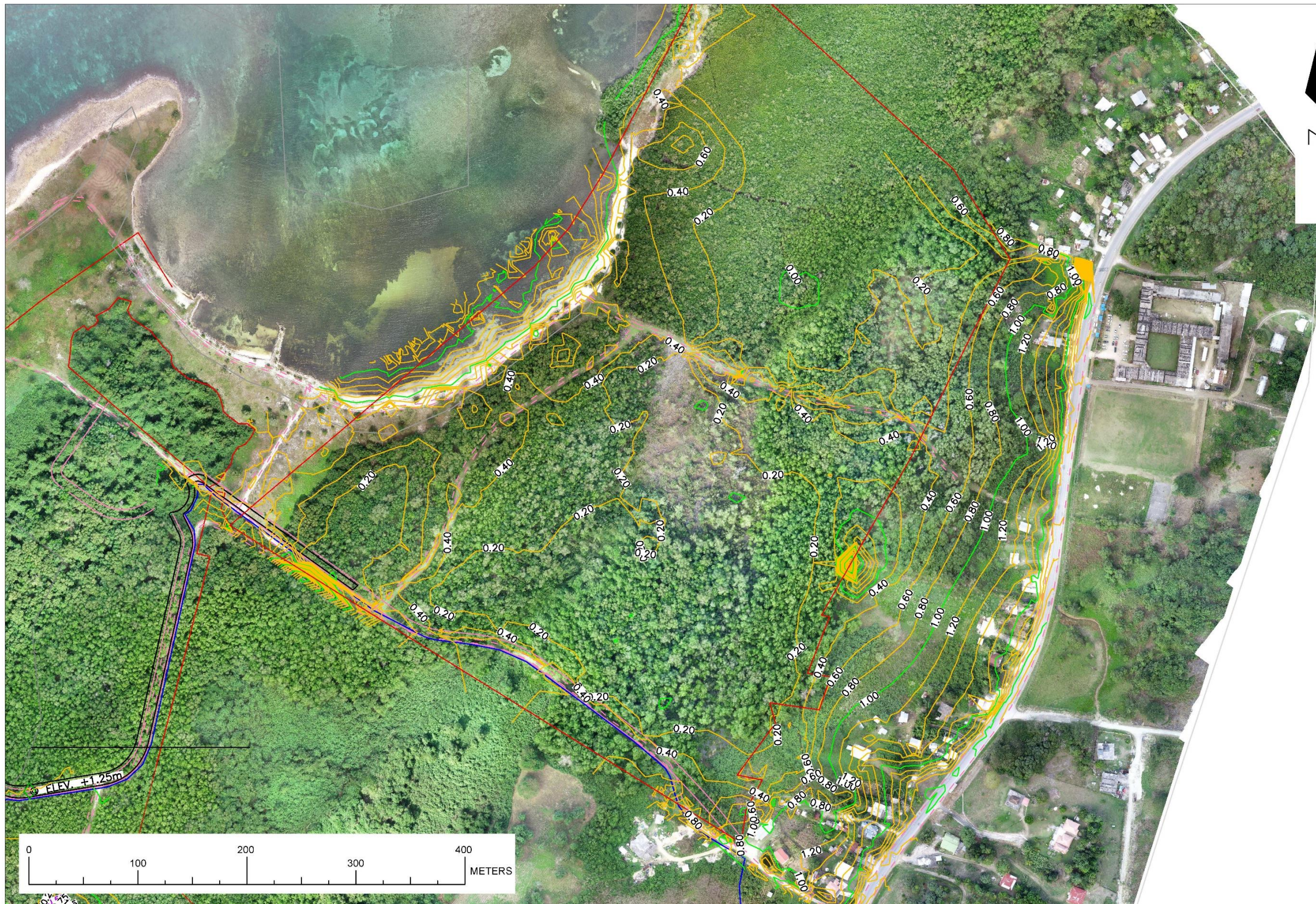
Figure 6-3 Topography at eastern section of property, highlighting identical elevations in mangrove forest (yellow circles)
