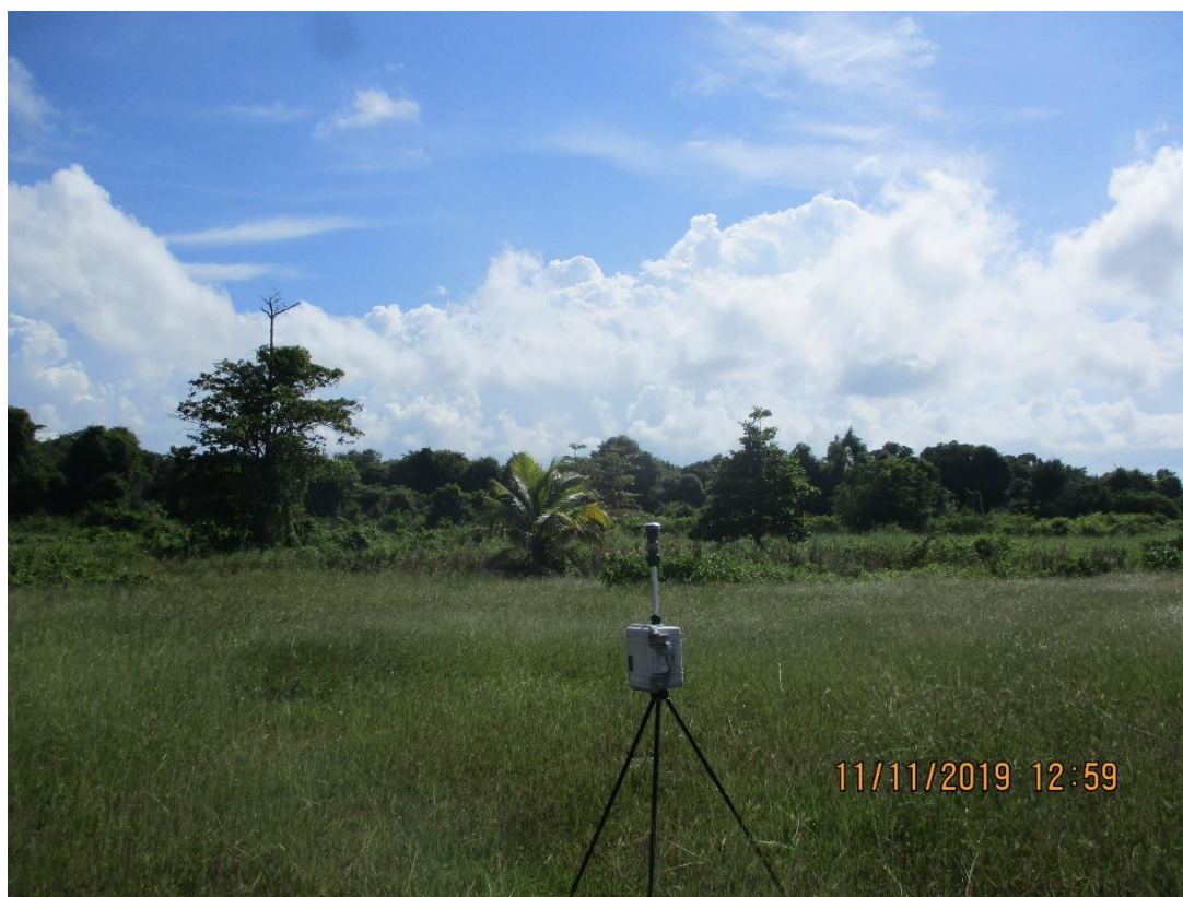
Plate 6-7 Particulate meter setup on site
