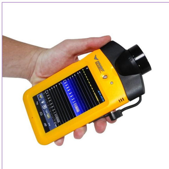
Plate 4-2 Anabat Walkabout bat detector
