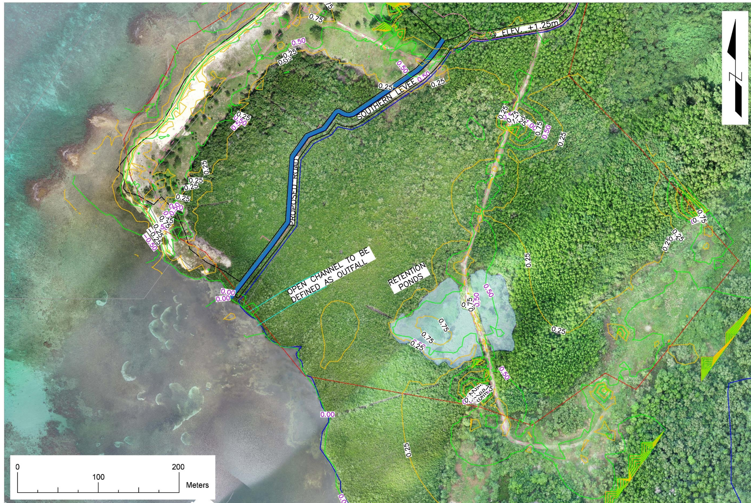
Figure 6-2 Western mangrove topography with proposed drainage ponds
