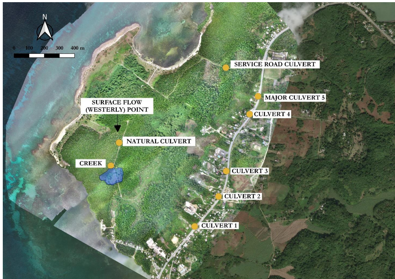
Figure 6-11 Culvert locations on highway and important drainage features on property
