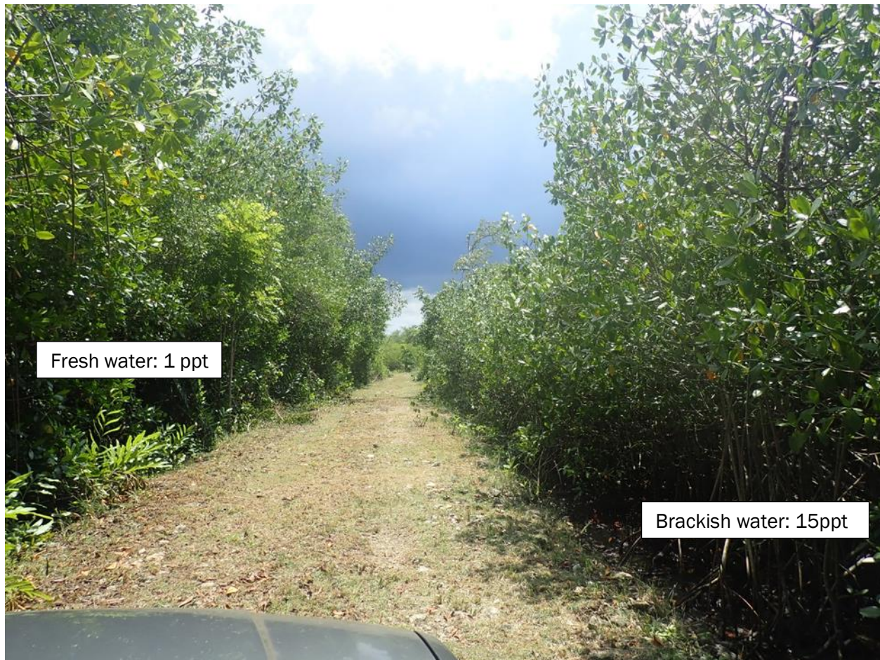
Plate 6-61 Segregation of fresh and saline/brackish water as a result of roadway Photo taken Nov 2019 showing salinity difference along Western access road
