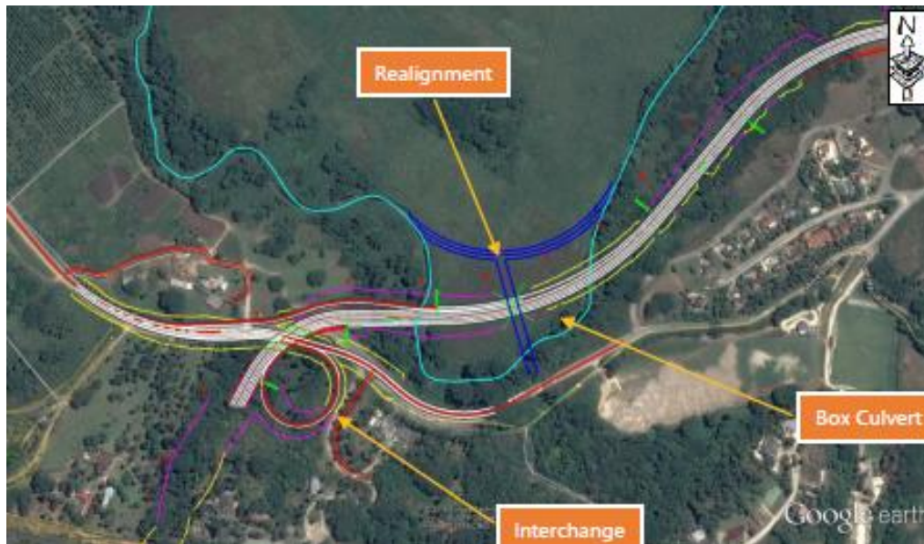
Figure 2-4 Proposed Montego River realignment and major box culvert for tributary crossing
