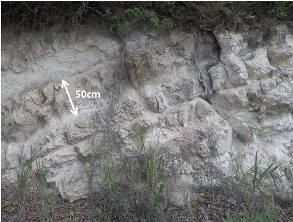
Plate 3-3 Montpelier Formation typical exposure along the Montego River consisting \frac{1}{2} to 1m thick beds of chawks and micritic limestone.
