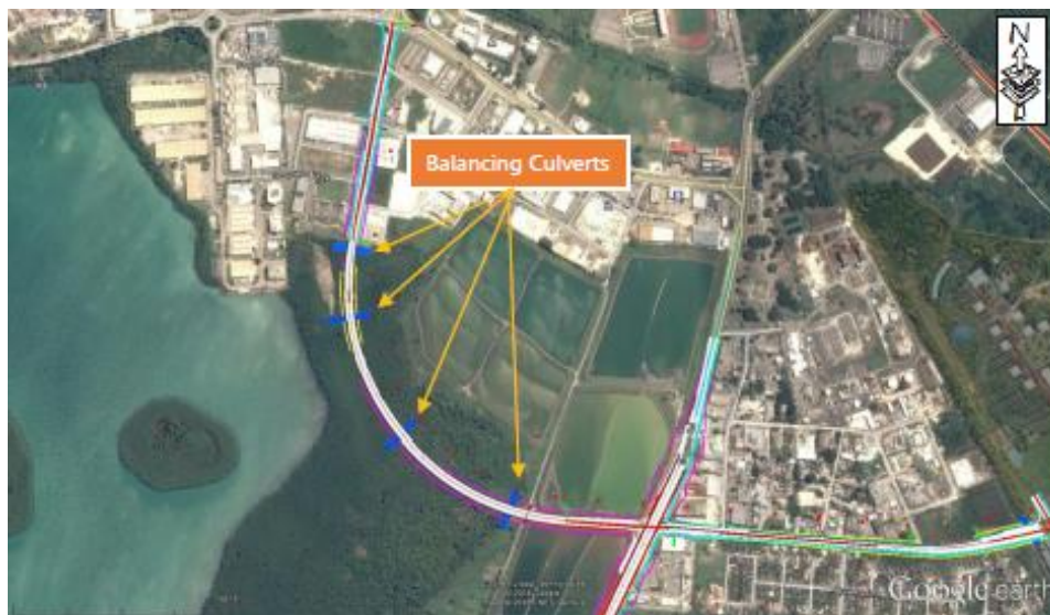
Figure 2-3 Placement of culverts in wetland area (CH 10+500 – 11+400)
