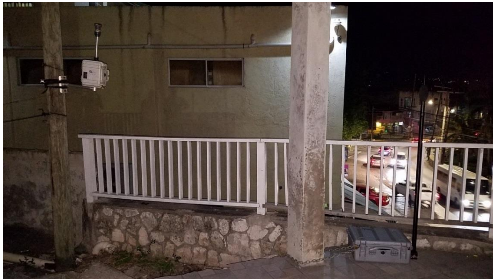
Plate 3-26 Photograph showing the Bruel & Kjaer noise meter and Airmetrics Minivol sampler at UTECH Caribbean School of Nursing Montego Bay, Campus on Barnett Street
