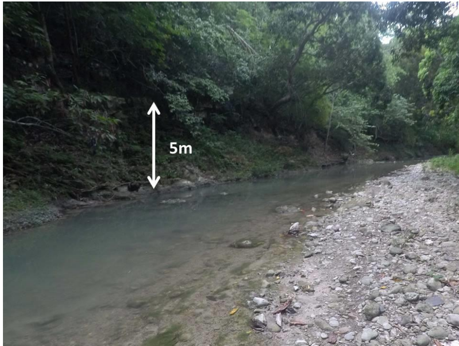
Plate 3-4 Montego River near milepost #17+100. Montpelier limestone exposed in the left bank of the river, coarse alluvial gravels on the right bank
