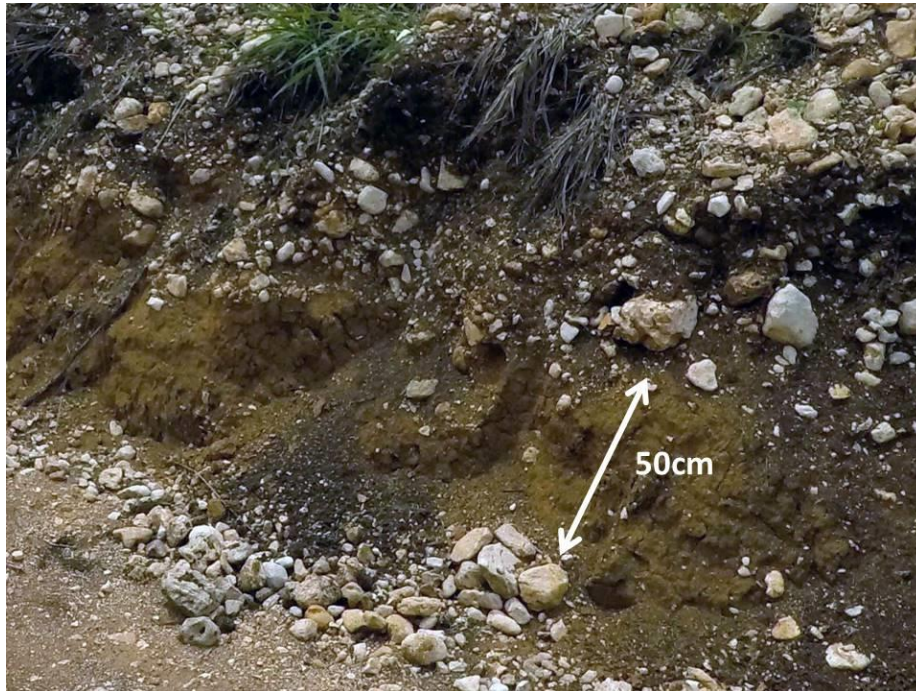
Plate 3-2 Quarternary Alluvium consisting of coarse calcareous gravels on top of layered sandy clay deposits near milepost #12+500
