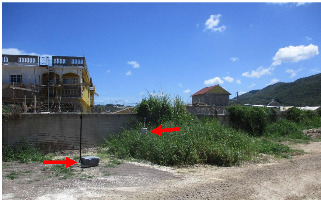
Plate 3-25 Photograph showing the Bruel & Kjaer noise meter and Airmetrics Minivol sampler at Station along Long Hill Bypass
