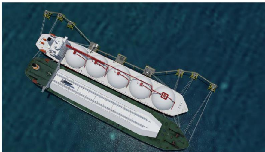
Figure 2: Proposed amendment – larger storage and regasification on FSRU and no terminal for regasification
