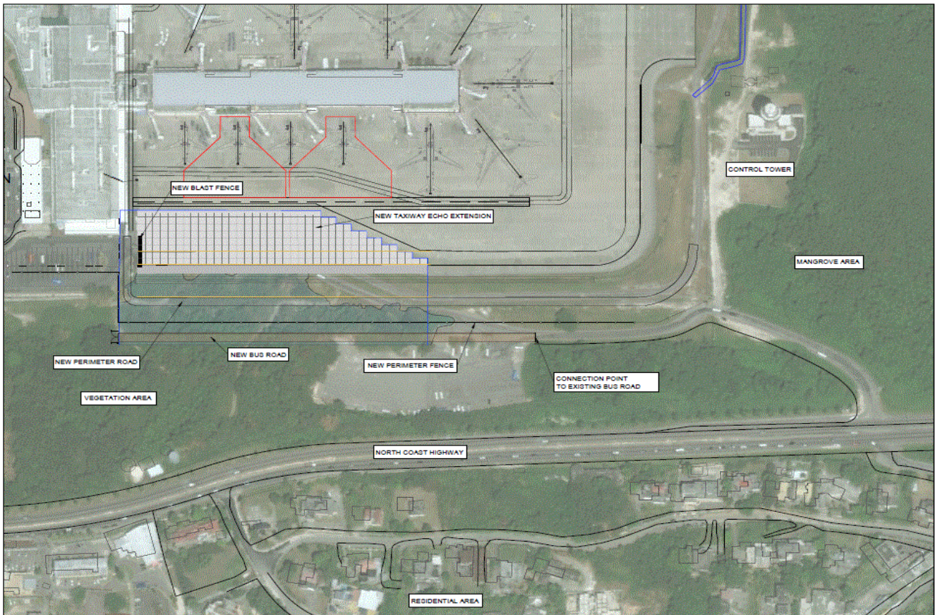
Figure 12: Proposed expansion of Taxiway Echo, as well as new bus road, perimeter road and fence
