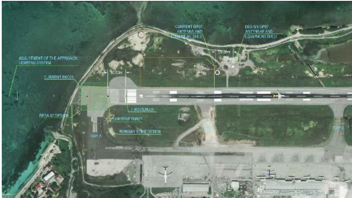
Figure 11: Proposed location for the RESA and relocation of thresholds and NAVAIDS at Runway 07 end (western end of runway)
