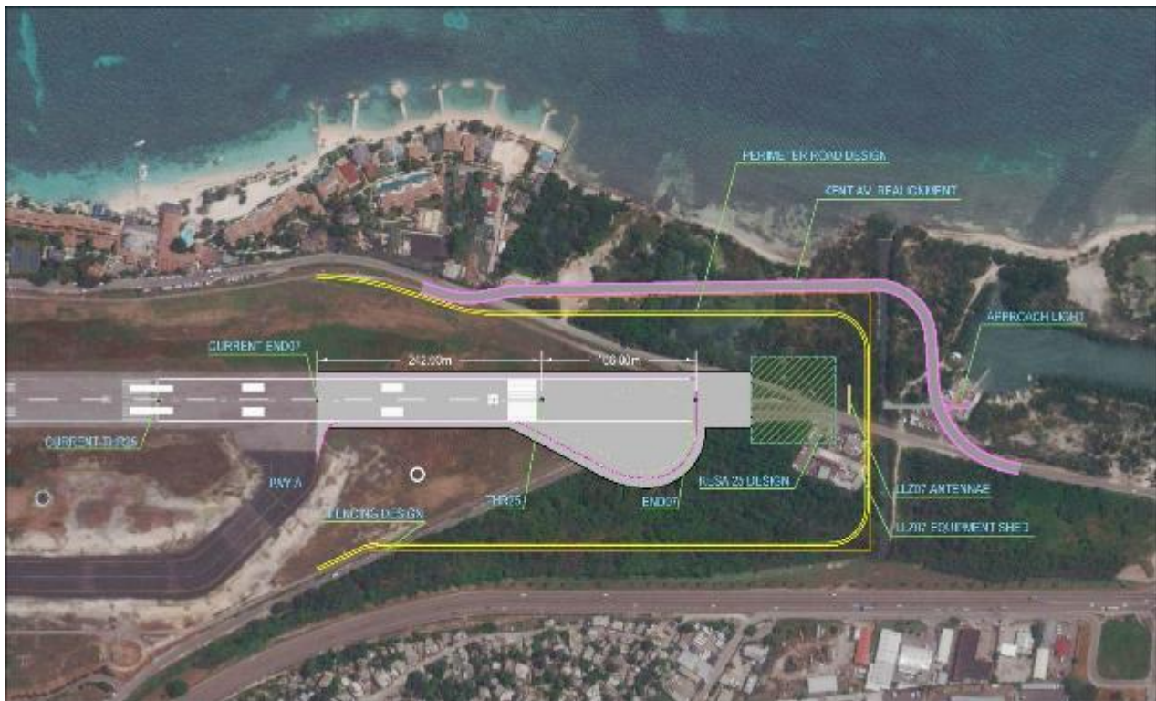
Figure 10: Proposed runway extension, establishment of RESA, and relocation of thresholds and NAVAIDS at Runway 25 end (eastern end of runway, Component 2, Component 3), along with the new perimeter road and fencing (Component 5)
