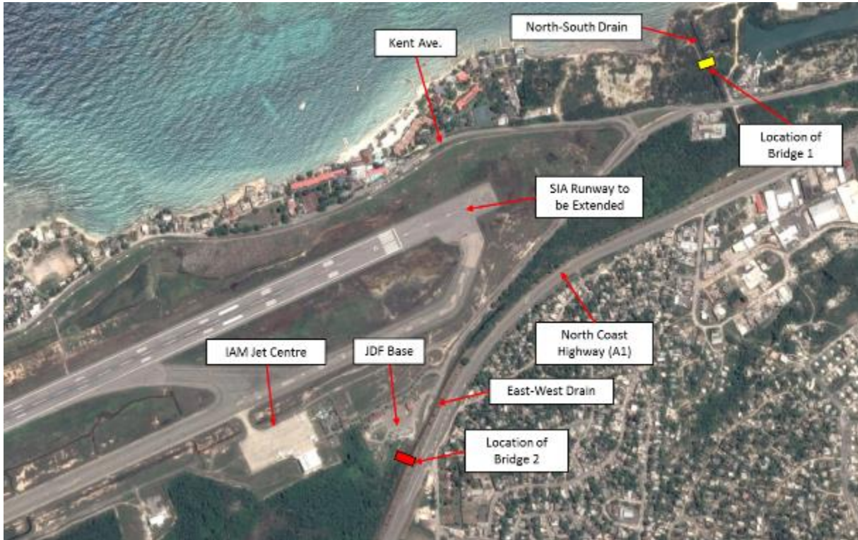
Figure 9: Project area and location of the proposed bridge across the large north-south drain on the realigned Kent Avenue (Bridge 1) and the proposed bridge from the North Coast Highway (A1) across the large east-west drain to access the JDF base and IAM Jet Centre (Bridge 2).
