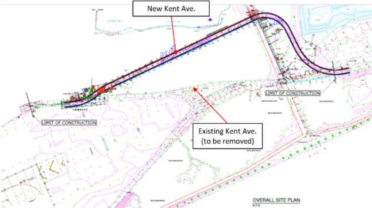
Figure 7: Overall site plan for Kent Avenue showing new and existing road alignment
