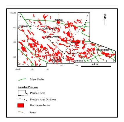
FIGURE 3-17: Fault Map of Jamalco of the Jamalco Mining Prospect Area in Manchester.<sup>1</sup>
