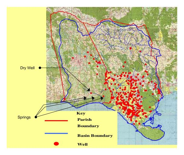
FIGURE 3-9: WELLS IN THE RIO MINHO HYDROLOGIC BASIN
