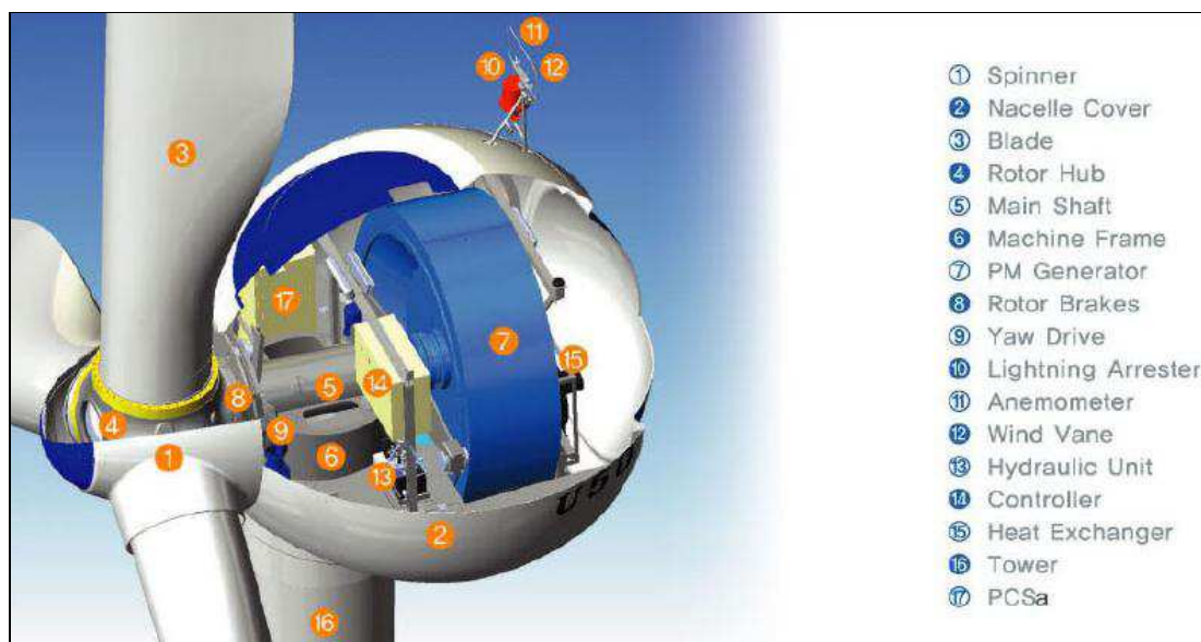
Figure 6 - Wind Turbine Components
