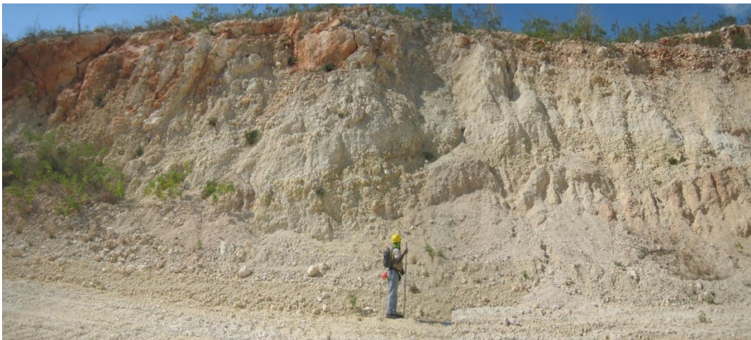
Plate 5.1.9: Another exposure of the rubbly and marly characteristics of the Newport Limestone near the t south eastern end of the project site
