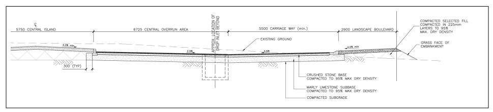
Figure 4 Part of Type I Road Section (Centre Island to Verge)
