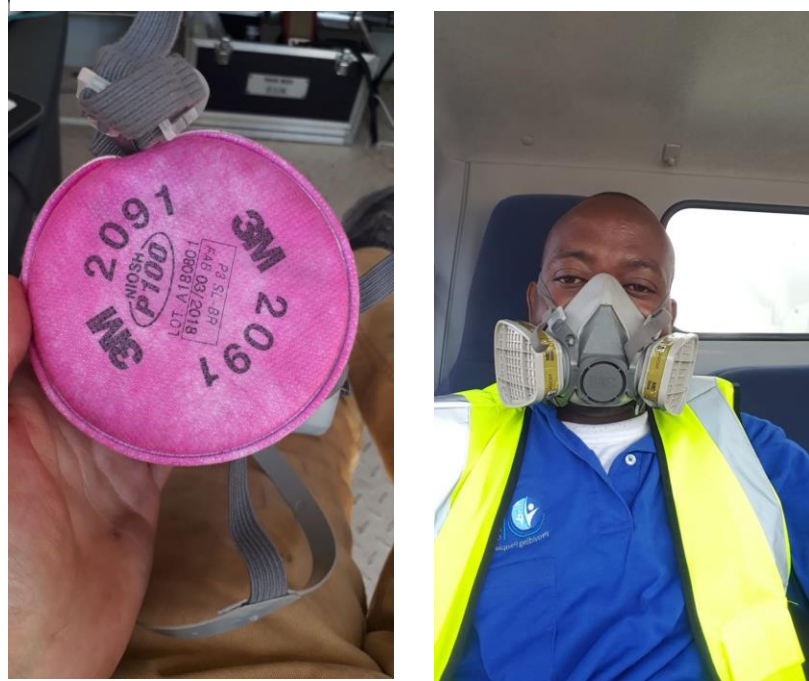
Figure 6 Respirator supplied to incinerator operators supplied with both particulate and multi-gas cartridges
