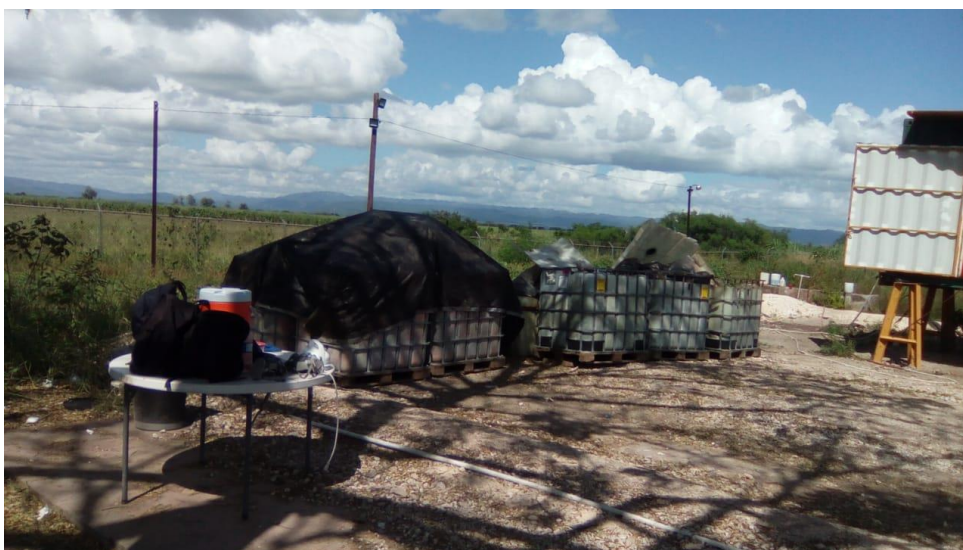
Figure 3.3 Modified IBC containers being used for Hazardous Waste Storage
