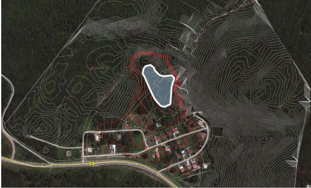
Figure 6.2.3: The 13 m contour no-fill zone (light blue polygon) for coral spring outlet sinkhole. Proposed post-development contour modifications are shown in red. White contours are the existing site contours. (Source: Richardson, 2012)
