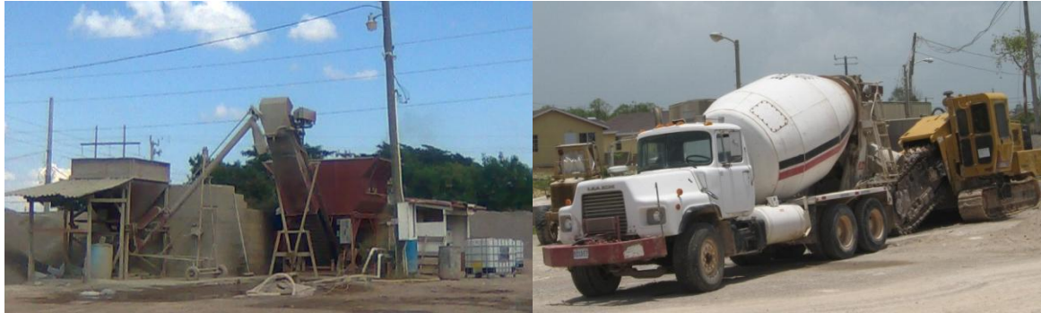
Plate 1.6.8a: Left - Concrete Batching Plant; Right – Mixer truck at a Concrete Batching Plant
