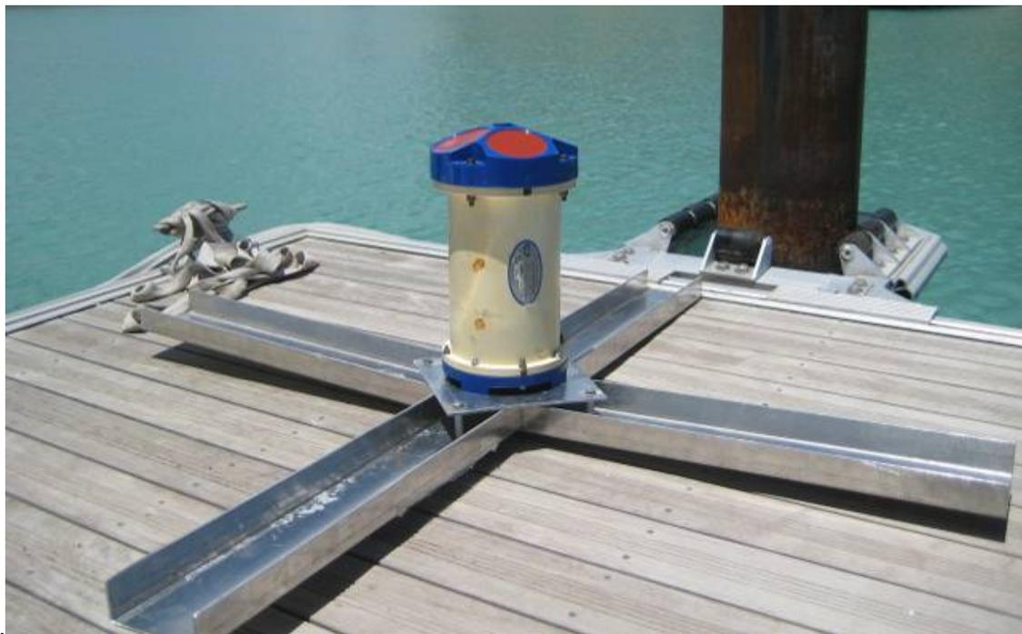
Figure 2.3 ADCP mounted on aluminium frame
