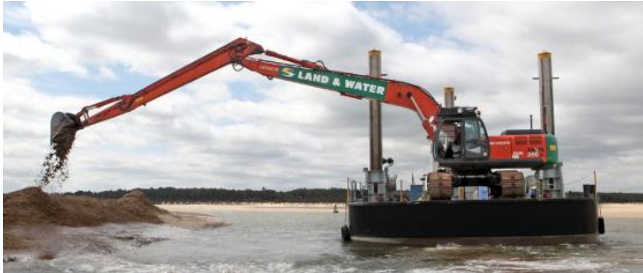
Plate 5-4 Example of a long-reach excavator with shaping bucket
