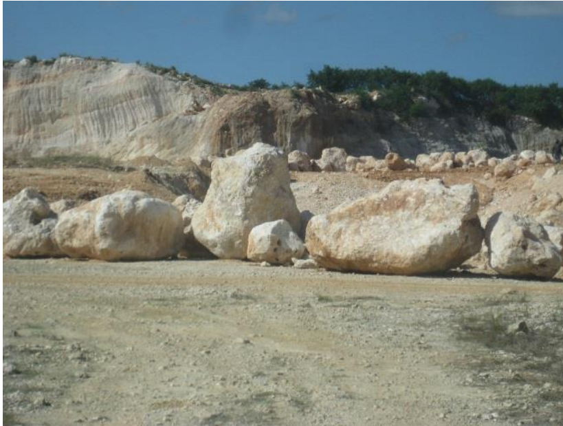
Plate 7-1 Clean quarried rocks washed and sorted on quarry floor
