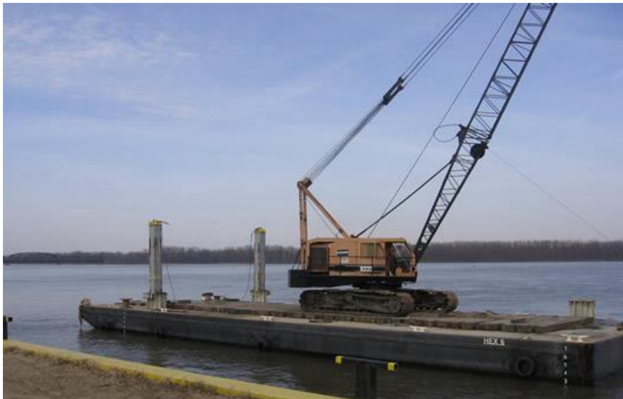
Plate 5-6 Spudded barge with crane
