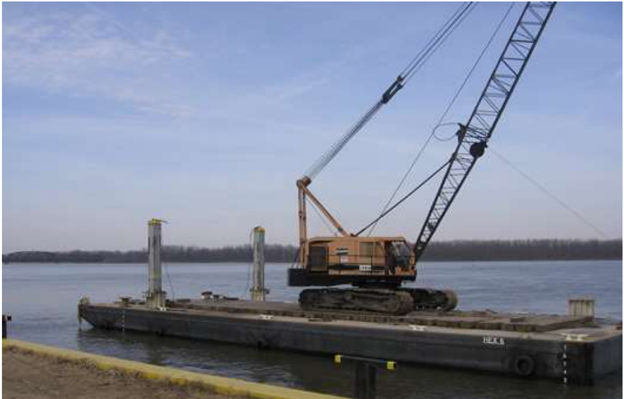
Plate 3-6 Spudded barge with crane
