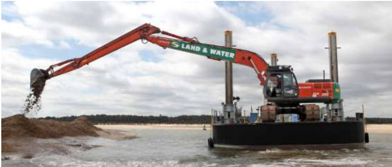
Plate 3-4 Example of a long-reach excavator with shaping bucket
