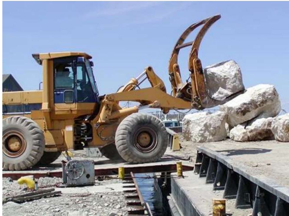
Plate 3-5 Retrieval of boulders using front end loader
