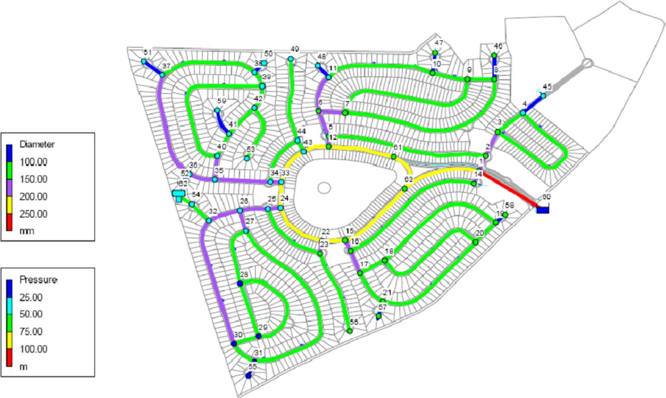
Figure 2-7: Water distribution model for the proposed Holland Estate Development - Preliminary Design Fire Flow
