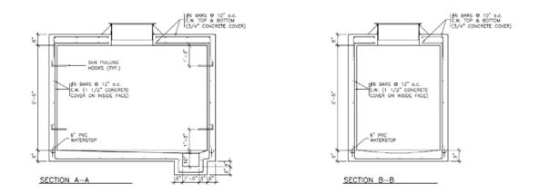
TYPICAL MANHOLE DETAIL - MARINE CABLE LANDING LOCATIONS SCALE  $1/2^{r}=1^{r}-0^{r}$
