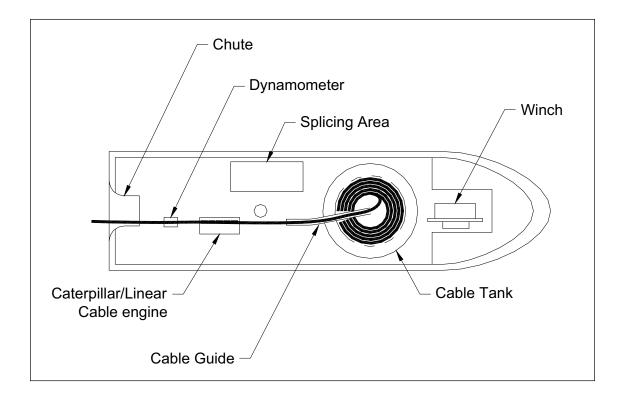
FIGURE 1-17: TYPICAL DECK LAYOUT
