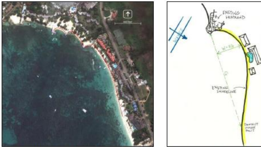
Figure B: The existing shoreline exhibits a weak crenulate shape south of the local headlands. In such shape, the shoreline is “indented” landward by some minor width ( W ) that is a function of the open shoreline length ( G ) down-wave of the headland. Filling the indentation with sand to straighten the shoreline (without stabilizing structures) results in rapid loss of the sand fill as the beach seeks to recover its embayment shape. For this reason, some modest level of structures is warranted at the site.
