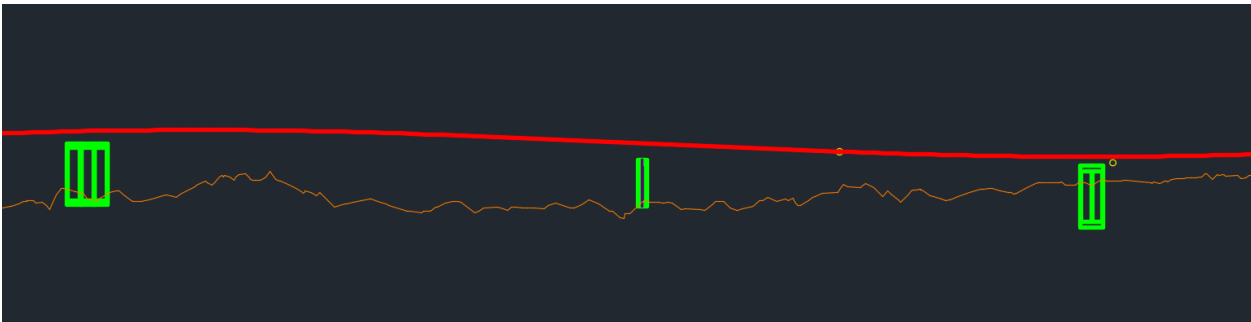
(b) Roadway profile showing raised roadway with box culverts
