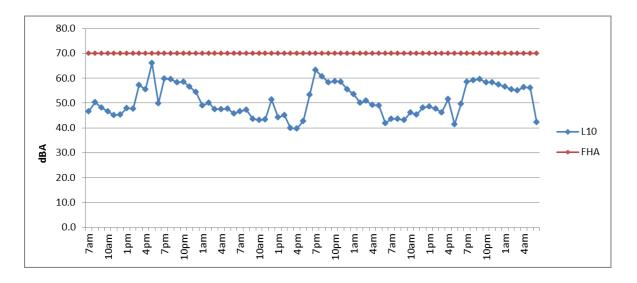
Figure 4.76 - Comparison of L10 at Station 4 with FHA standard
