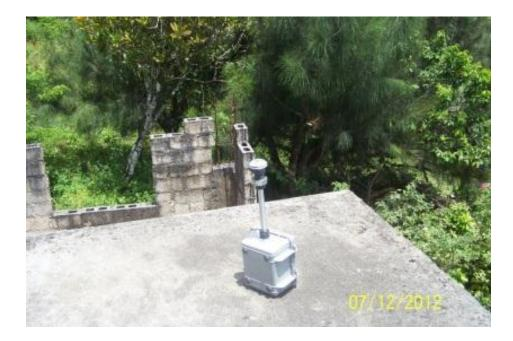
Plate 4.17 – Photo showing particulate sampler
