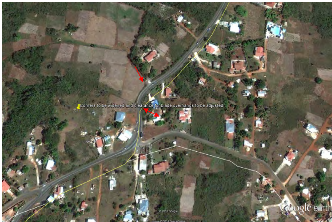
Fig 122. Adjustments to be made to corners to allow wheel base clearance and tail swing. Kinkead Junction Main road prior to arriving in town of Junction.
