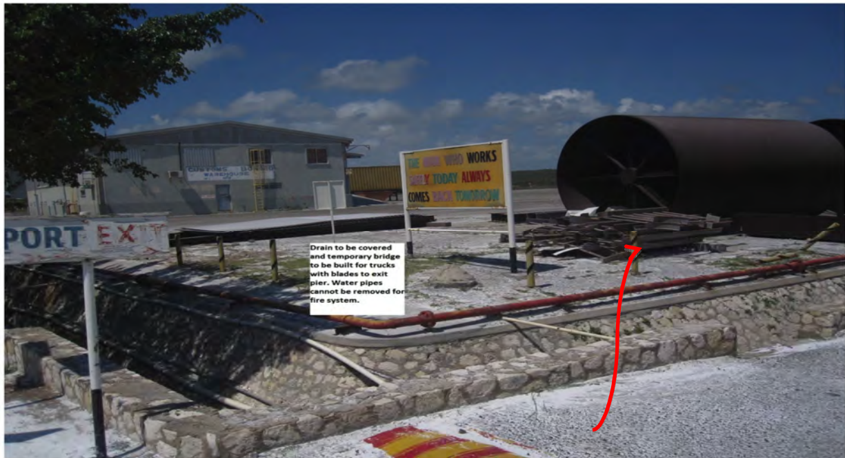
Fig 7. Option for clearance to allow exit of blades from port - A temporary bridge must be constructed to pass over an existing waterway and the removal and replacements of signs.
