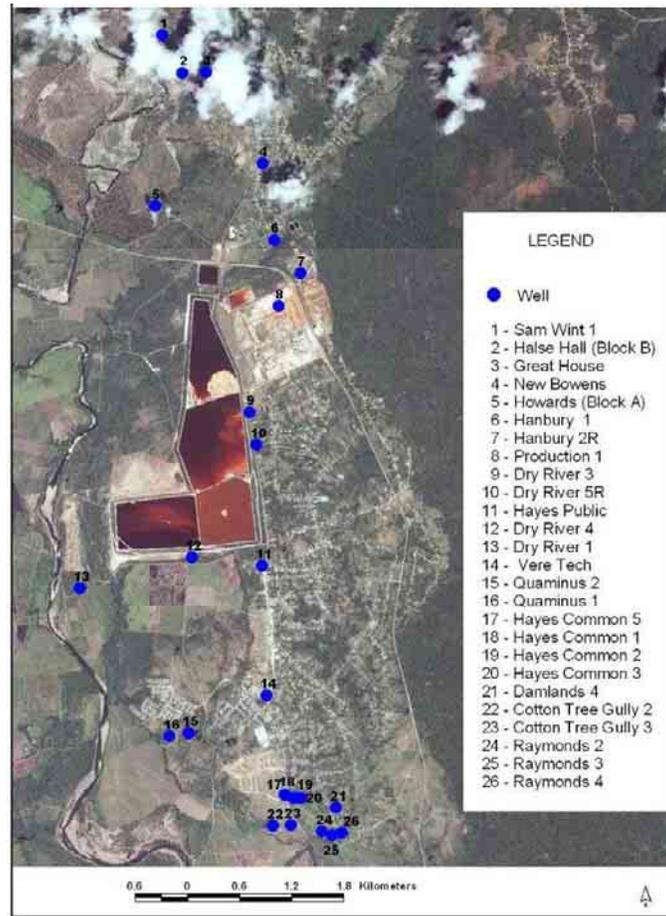
The greater numbers of the wells is located south of the REFINERY, are all owned by SCOJ, are all used for irrigation and are centered on the Hayes Common-Raymonds area. The location of these wells is along the South Coastal fault that is open to the sea at the western and eastern ends. The high permeability associated with the fault and the ponding of groundwater behind the fault influenced the locations. The wells located along the fault are high producers.
