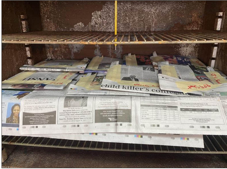
Plate 4-11 Labeled above and below ground vegetative components per site in Despatch LDB Lab Oven
