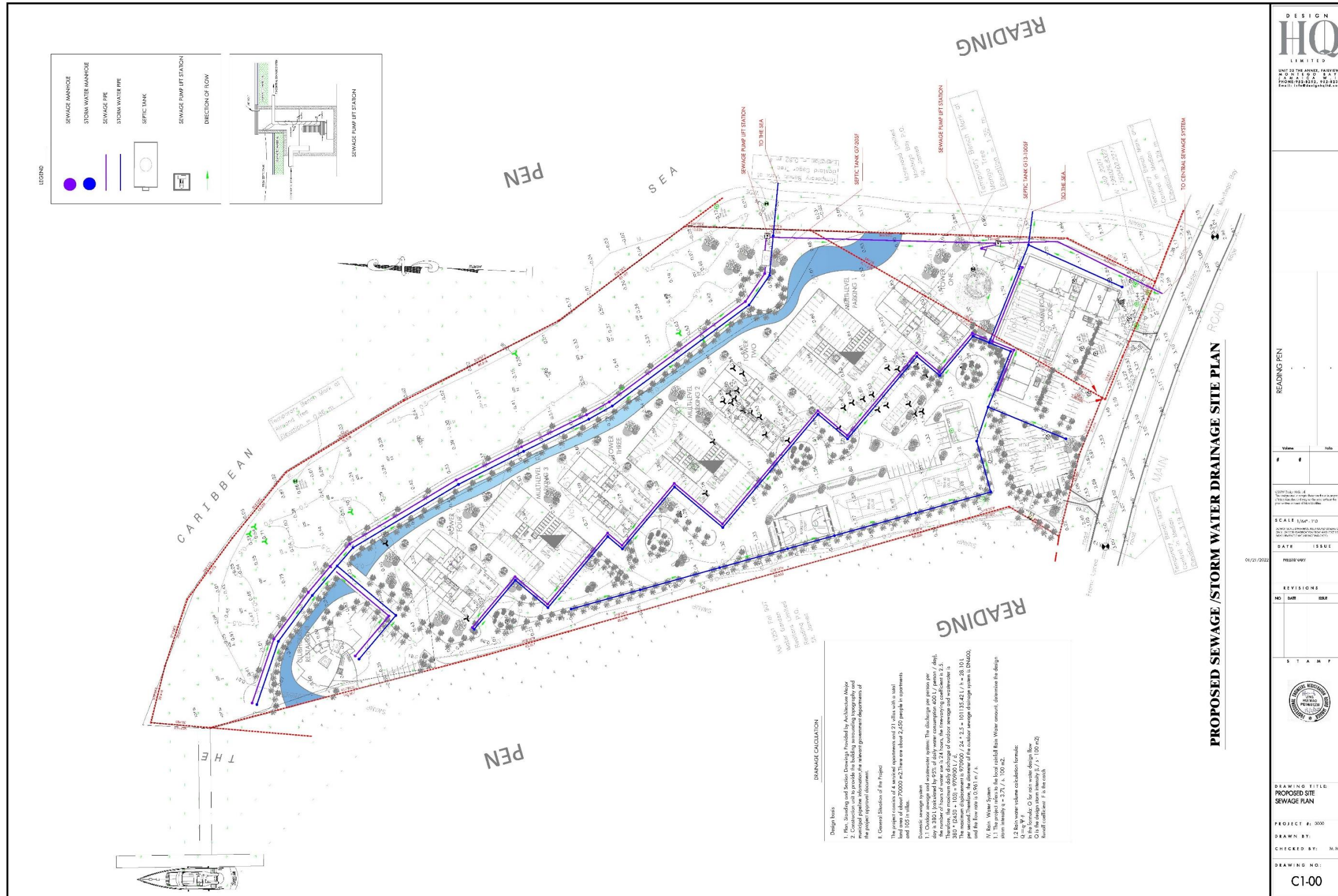
Figure 3-9 Proposed sewage and storm water drainage system
