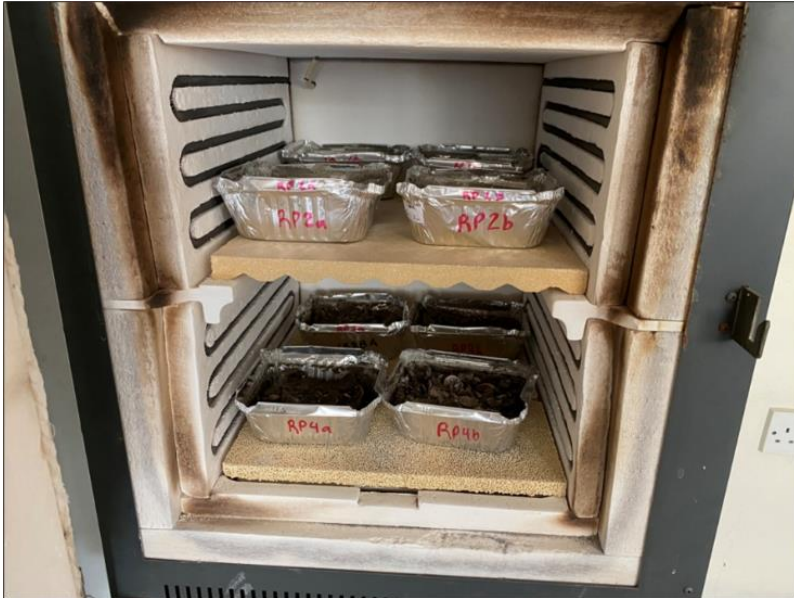
Plate 4-13 Muffle Furnace containing soil samples recovered from core samples within the Reading Pen peninsula
