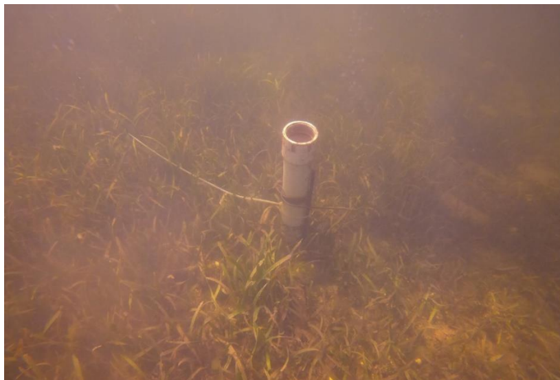
Plate 4-1 An example of the Sediment Trap deployed
