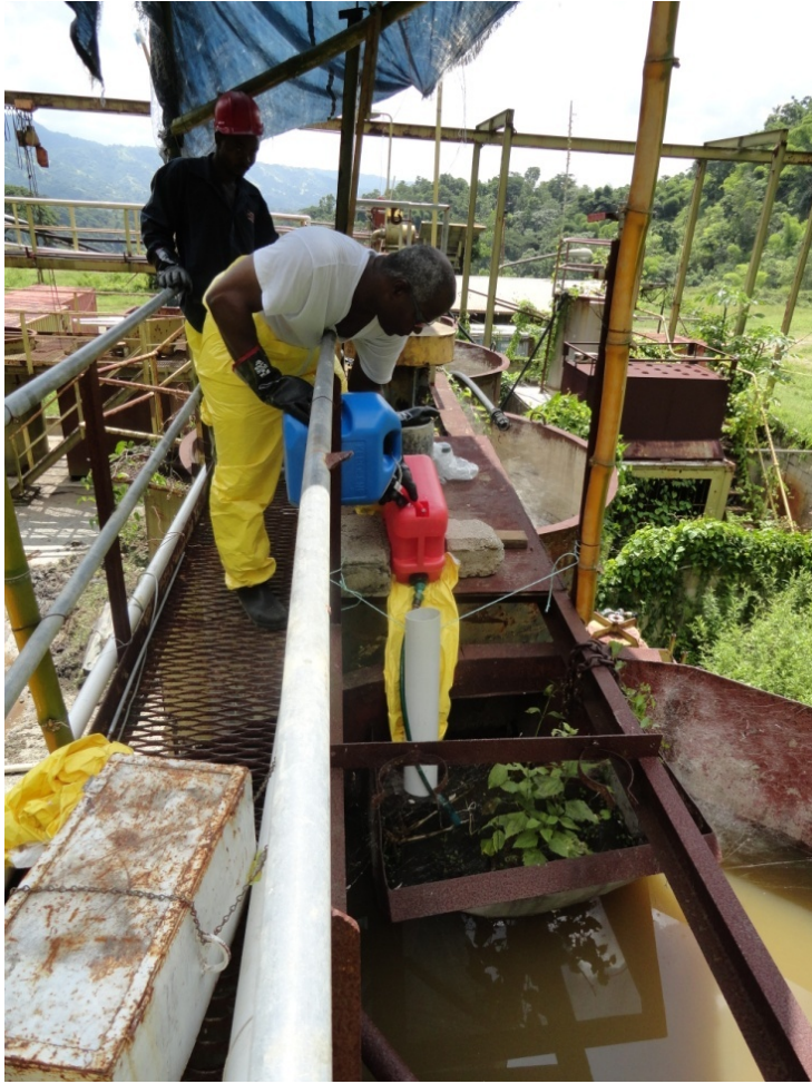
Plate 10 Photo showing subsequent H 2 O 2 addition process (July 21, 2011)
